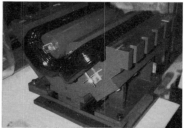
Fig. 5 Prototype of quadrupole magnet under construction.
