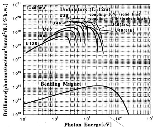
Fig. 2 Brilliances of 12 m undulators with typical periods and the bending magnet.
