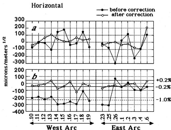
Fig. 6 The coefficients  $a$  and  $b$  of the fit for the horizontal leakage orbits of the first (before correction) and the second (after correction) measurement. The bumps are named by the target magnets. The strength of the targets was changed by the data fitted  $b$  of the first measurement. If the target deviates 0.2%, it produces  $b$  component leakage orbit of 50 microns/meter<sup>1/2</sup>. This and the level of 1% target error are shown as the horizontal line in the bottom figure.
