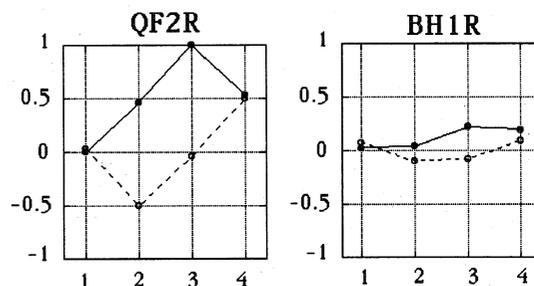
Fig. 4 Values of  $W_a$  (dotted line) and  $W_b$  (solid line) at QF2R and BH1R magnets in the horizontal  $\pi$ -bump. The magnets are numbered from upstream to downstream. The values of  $W_a$  and  $W_b$  are normalized by the  $W_b$  at the third QF2R magnet. This magnet, which locates almost the center of the bump region, has the maximum weight in the summation for  $b$ .
