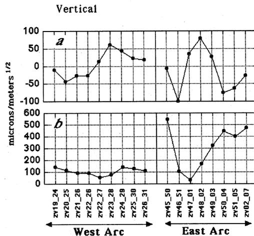
Fig. 3 The observed coefficients  $a$  and  $b$  of leakage orbits for the vertical bumps in West and East Arc. The bumps are named by the correctors to produce it.
