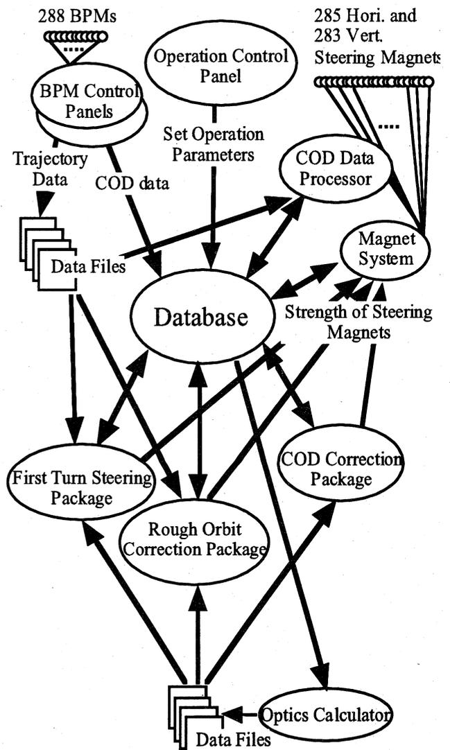
Fig. 1 Composition of orbit correction system.
