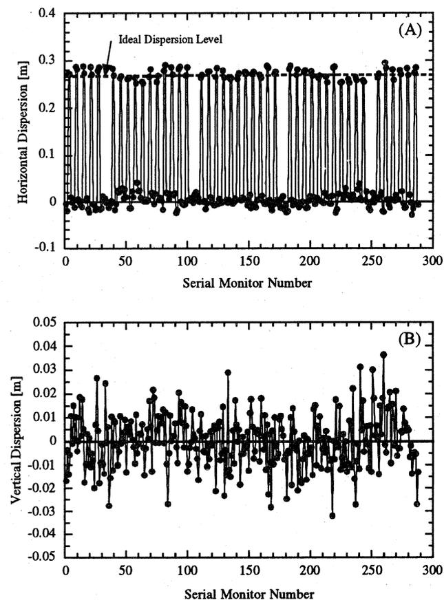
Fig. 5 Dispersion measured after the COD correction. The upper right symbols (A) and (B) denote respectively a horizontal and a vertical planes.
