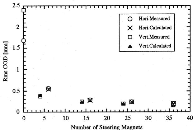
Fig. 4 Comparison between measured and expected rms values of the COD after the correction. The number of steering magnets represents the simple sum of the number used in each correction step.
