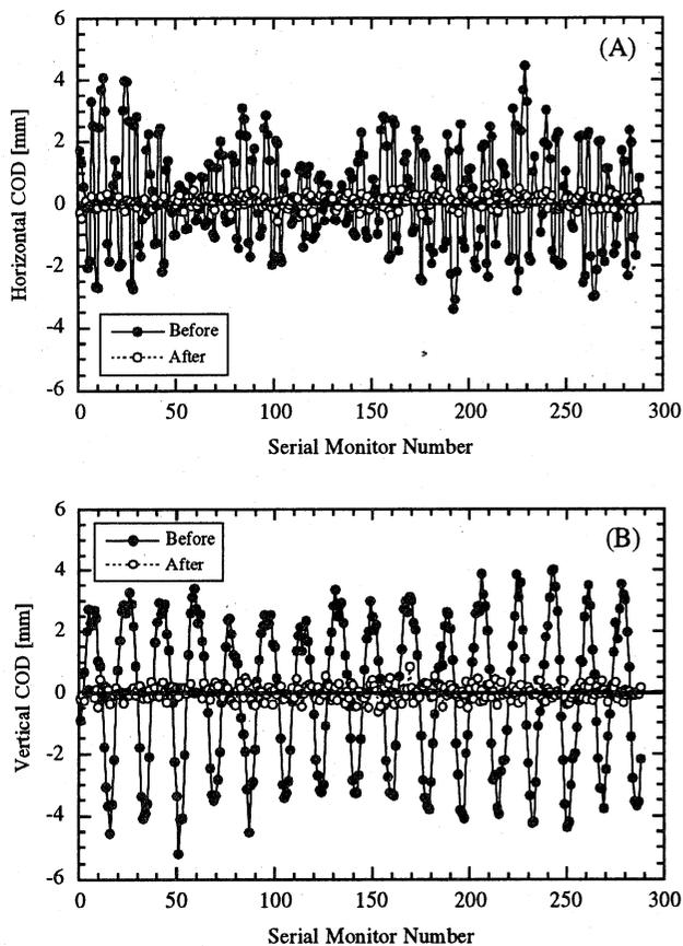
Fig. 3 COD before and after the correction. The upper right symbols (A) and (B) denote respectively a horizontal and a vertical planes.
