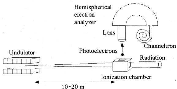
Fig. 2 Schematic drawing of the absolute measurement of undulator brightness by use of a hemispherical electron analyzer.
