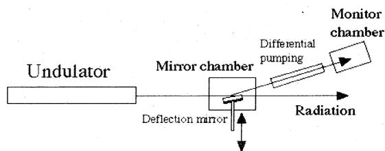
Fig. 1 Schematic drawing of the undulator beamline for absolute measurement of radiation intensity by photoionization of a rare gas.
