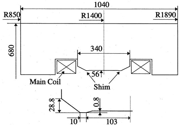
Fig. 3 Cross-sectional view of the conventional shim-type magnet
