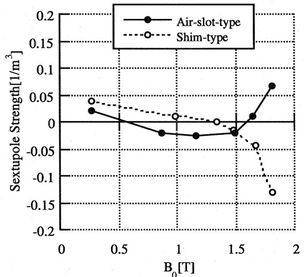
Fig. 6 Dependence of calculated sextupole strength on magnetic field strength,  $B_0$ , at design orbit
