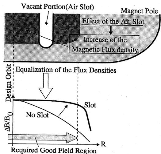
Fig. 1 The scheme of improvement of magnetic field distribution by introducing air slots into the magnet pole
