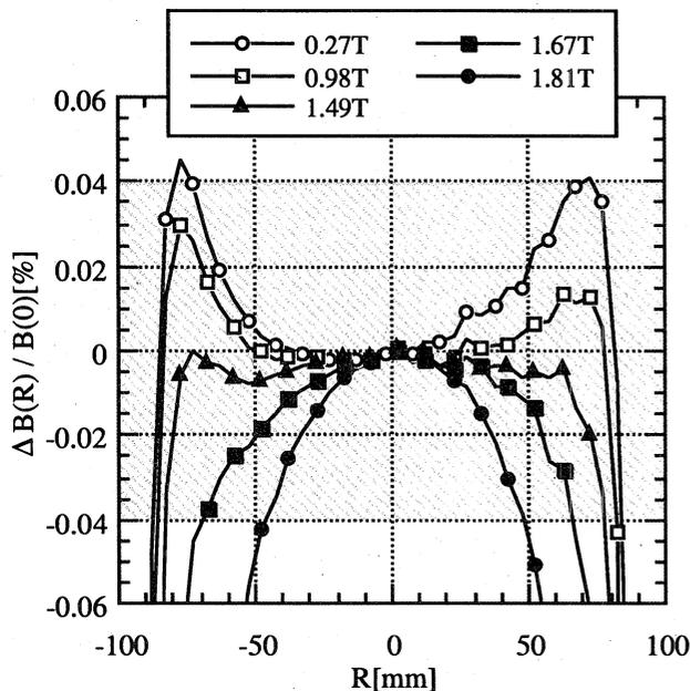
Fig. 5 Two-dimensional magnetic field distribution of the conventional shim-type magnet
