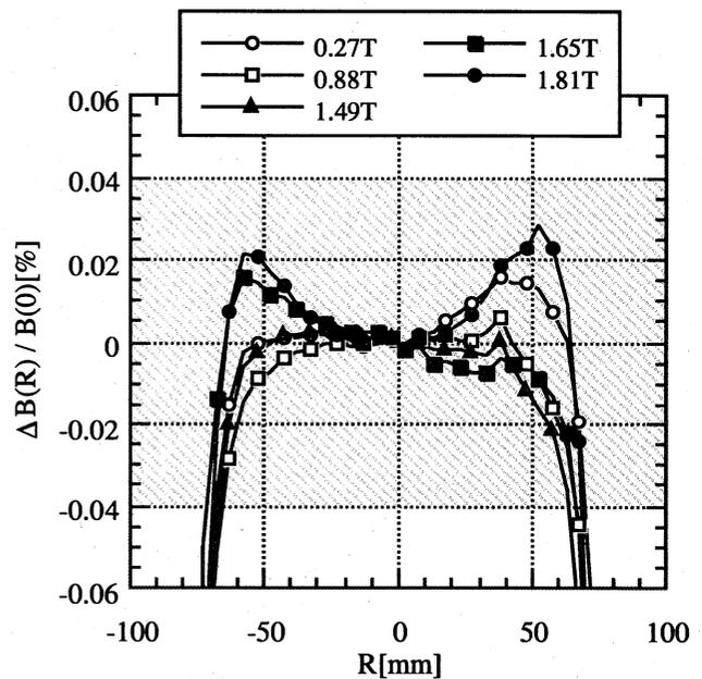
Fig. 4 Two-dimensional magnetic field distribution of the Air-slot-type magnet
