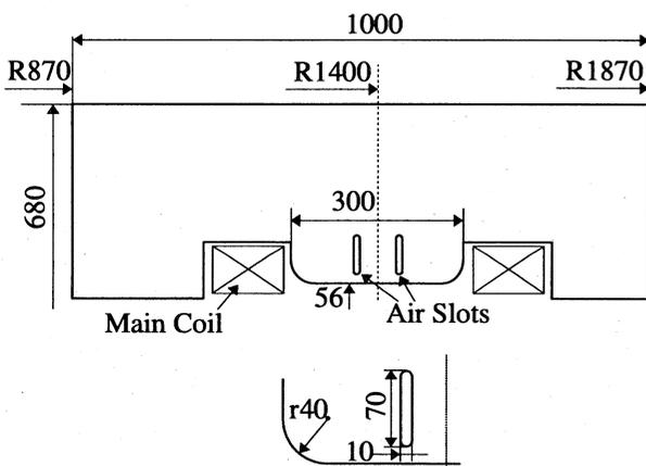
Fig. 2 Cross-sectional view of the air-slot-type magnet
