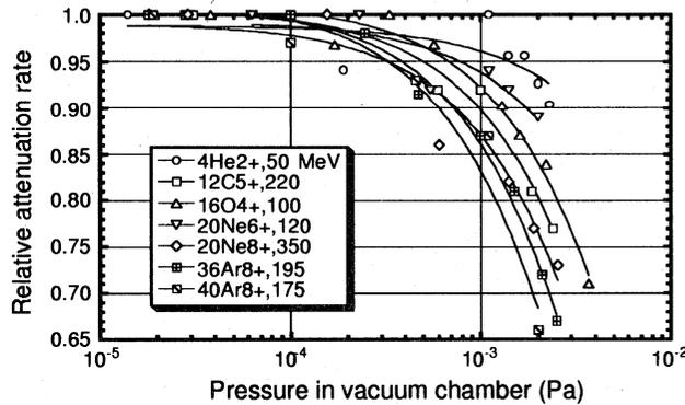
Fig. 8 The beam attenuation for various ions in the injection line.
