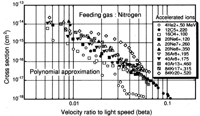
Fig. 9 Typical charge exchange cross sections estimated based on beam attenuation.
