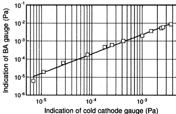
Fig. 5 A calibration line for cold cathode gauge used in experiment.
