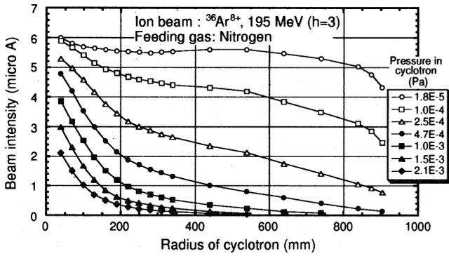
Fig. 6 The beam attenuation for  $^{36}\text{Ar}^{8+}$ , 195 MeV ion by nitrogen gas feeding into the vacuum chamber.
