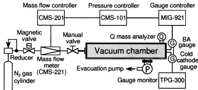
Fig. 3 A block diagram for pressure control in the vacuum chamber of the cyclotron.
