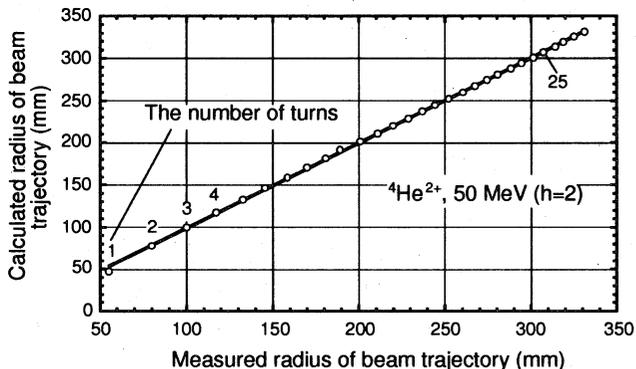
Fig. 2 A relationship between calculated and measured radii of the beam trajectory.
