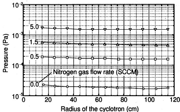
Fig. 4 Pressure distributions along the radius of the cyclotron.
