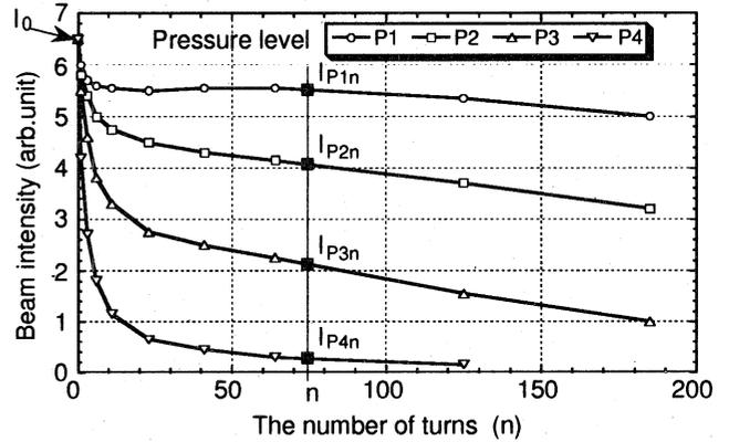
Fig. 1 A calculation model for attenuated beam intensities by gas feeding.
