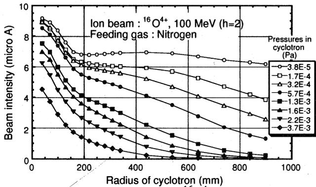
Fig. 7 The beam attenuation for  $^{16}\text{O}^{4+}$ , 100 MeV ion by nitrogen gas feeding into the vacuum chamber.
