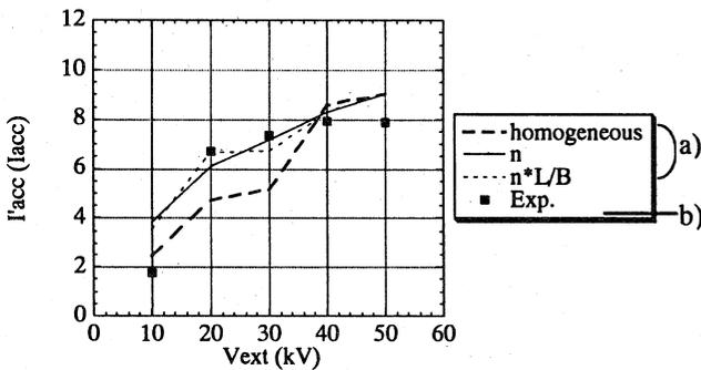
Fig. 7 Experimental and calculation results of  $V_{ext} - I_{acc}$  ( $M2=700A$ ,  $d_{ext}=40mm$ ,  $I_{total}=9mA$ )
