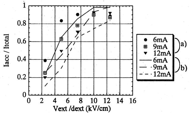
Fig. 5 Calculated dependence of  $I_{acc}$  on  $V_{ext}$  for different values of  $I_{total}$  together with the experimental data
