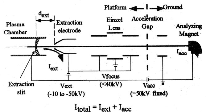
Fig. 1 A layout of the extraction system of NIRS-HEC ion source
