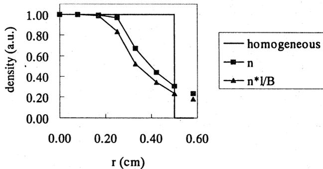
Fig. 6 Flux density distribution by TrapCAD
