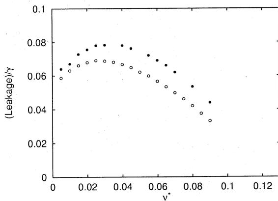
Fig. 4 Normalized leakage power from the beam splitter of Michelson FEL:  $\rho^* = 0.01$  ( $\circ$ ),  $\rho^* = 0.1$  ( $\bullet$ )
