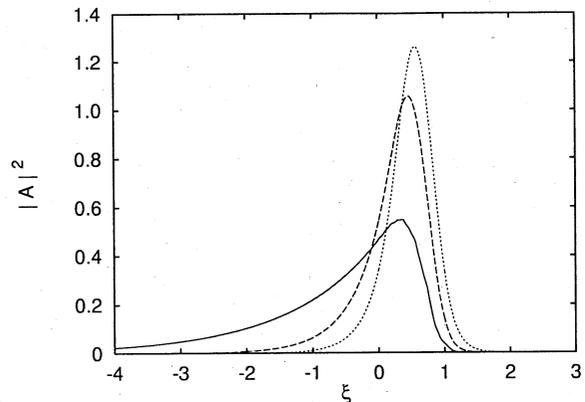
Fig. 5 Laser field profile for Michelson FEL with parameters:  $\rho^* = 0.01$ ,  $\alpha = 0.05$ ,  $\nu^* = 0.075$  (continuous line),  $\nu^* = 0.025$  (dashed line),  $\nu^* = 0.01$  (dotted line).
