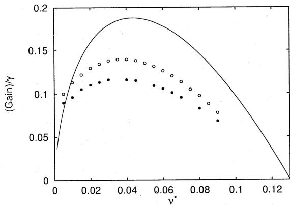
Fig. 3 Small signal gain for Michelson FEL ( $\delta_1 \delta_2 < 0$ ) vs equivalent cavity detuning:  $\rho^* = 0.01$  ( $\circ$ ),  $\rho^* = 0.1$  ( $\bullet$ ), the first supermode for FEL with conventional resonators (solid line).
