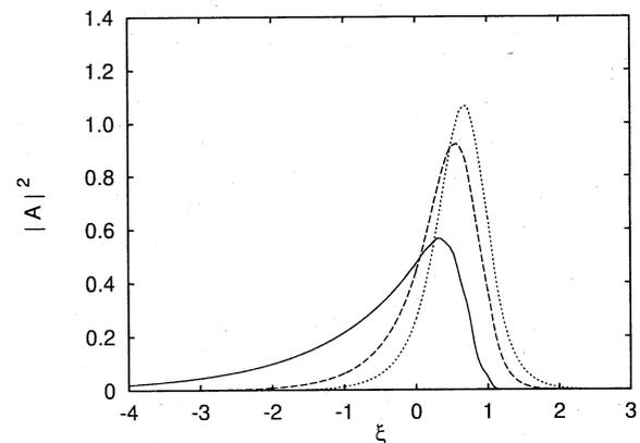
Fig. 6 Laser field profile for Michelson FEL with parameters:  $\rho^* = 0.1$ ,  $\alpha = 0.05$ ,  $\nu^* = 0.075$  (continuous line),  $\nu^* = 0.025$  (dashed line),  $\nu^* = 0.01$  (dotted line).
