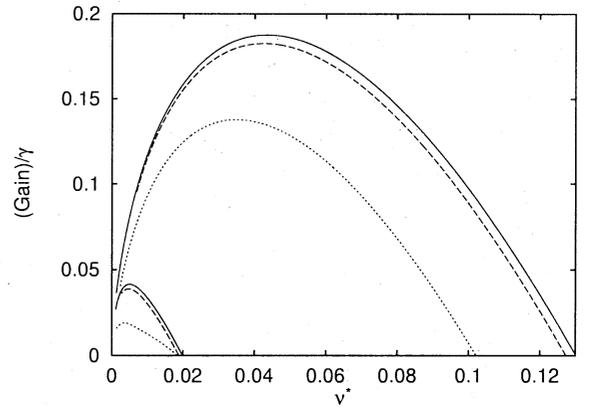
Fig. 2 Small-signal gain of the first two supermodes in Michelson FEL ( $\delta_1 > 0$ ,  $\delta_2 > 0$ ) vs equivalent detuning:  $\rho^* = 0.01$  (dashed line),  $\rho^* = 0.1$  (dotted line), conventional resonators (continuous line).
