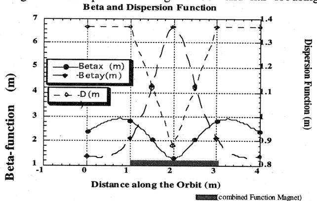
Fig. 2 Beta and dispersion functions for one superperiod.
