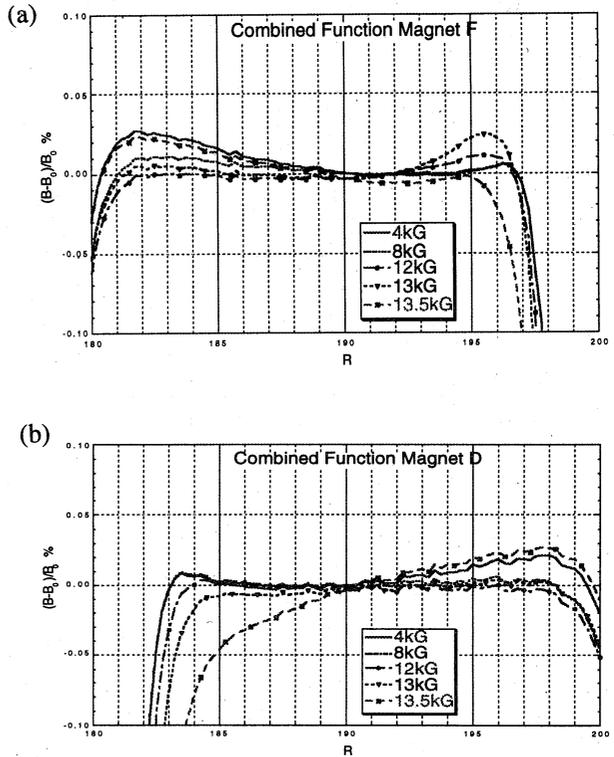
Fig. 4 Calculated Field Distribution in F (a) and D (b) sectors.
