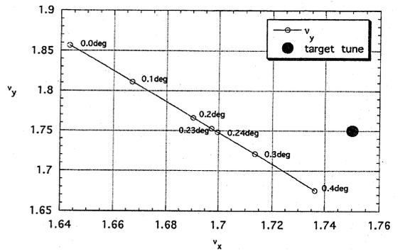
Fig. 7 Estimated betatron tune from field distribution. central orbit in the transition region between F and D sectors obtained with the three dimensional calculation is shown.
