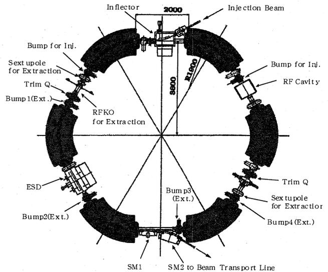
Fig. 1 Combined Function Proton Synchrotron.
