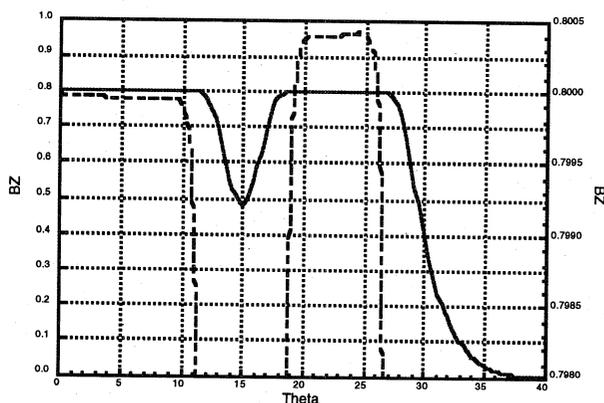
Fig. 6 Field variation along the central orbit in the transition region between F and D sectors..
