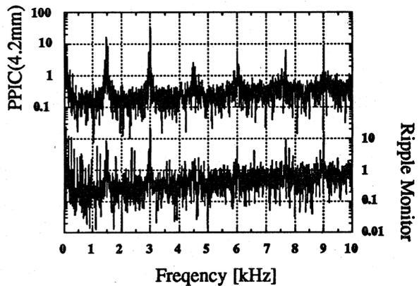
Fig. 5 Frequency spectra of the signals from the PPIC (4.2 mm) with the 758.8 Torr-air (upper) and the Ripple Monitor (lower). The repetition rate of the frequency modulation of RF-KO field is 3 kHz.
