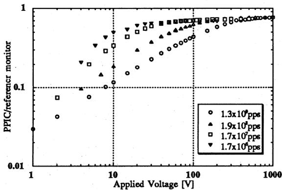
Fig. 3 The plateau curve of PPIC (3 mm gap distances) with 759.6 Torr-air for the beams of C<sup>6+</sup> (290 MeV/u). The frequency modulation of RF-KO is 777 Hz. The ordinate is the ratio between the output charge from the PPIC and the reference monitor.
