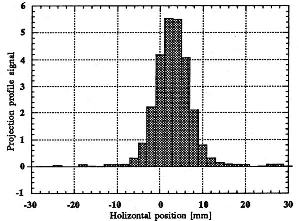
Fig. 7. The preliminary results of  $\text{C}^{6+}$  (290 MeV/u) beam profile. The beam intensity is  $4 \times 10^8$  pps. The applied voltage of MuSIC is 500 V.
