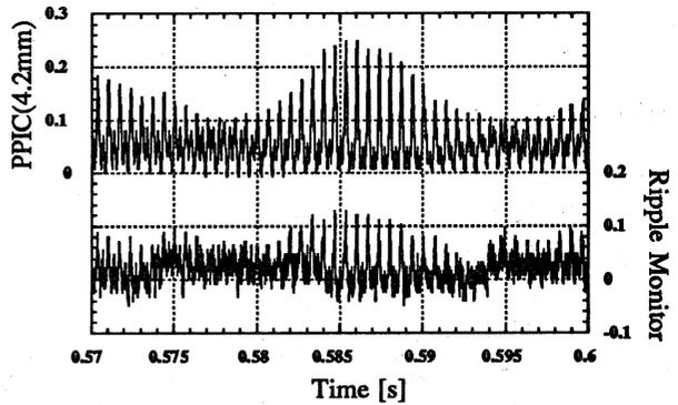
Fig. 4 Time structure measured by the PPIC (4.2 mm) with the 758.8 Torr-air (upper) and the Ripple Monitor (lower). The beam intensity is  $5.7 \times 10^8$  pps C<sup>6+</sup> (290 MeV/u) and the frequency modulation rate of RF-KO field is 3 kHz.
