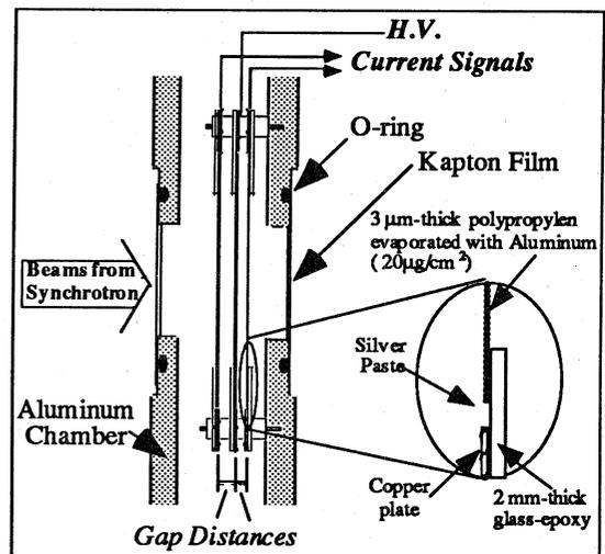
Fig. 1 The cross sectional view of the PPIC.
