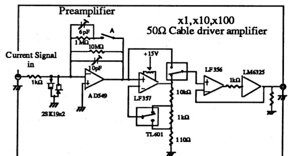
Fig. 2 The trans-impedance amplifier system. It consists of 10/100 M $\Omega$  pre-amplifier and x 1, x 10, x 100 Cable driver amplifier.
