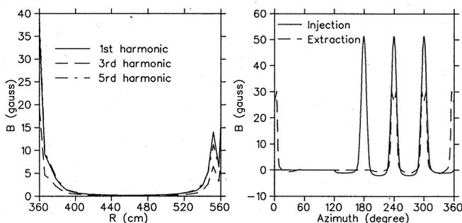
Fig. 3 Right: azimuthal distribution of the stray fields. The amplitude is 50 gauss at the radius of 370 cm, and 30 gauss at 550 cm. Left: Fourier components of the stray field as a function of radius.
