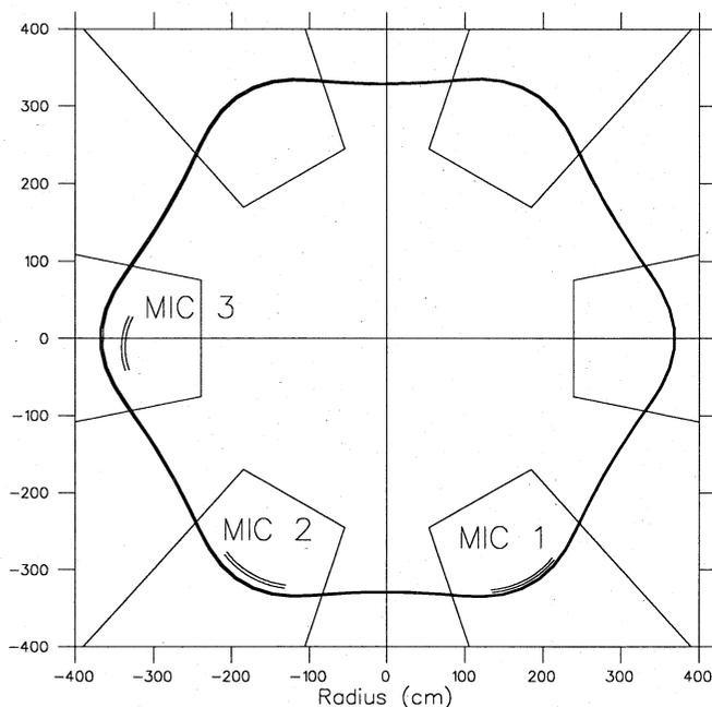
Fig. 5 Trajectory of inner radius of a finite emittance beam for the first five turns. The beam clears the MIC 1 which is located nearest to the beam.
