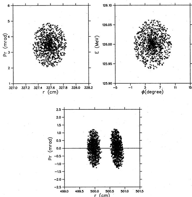
Fig. 2 Upper: the initial radial and longitudinal phase spaces which are coupled. Lower: the final radial phase spaces of the last two turns in front of the EDC.
