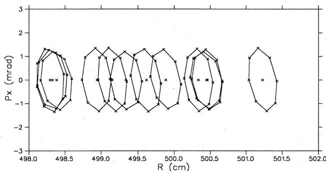
Fig. 4 Radial phase spaces for the last few turns. The last turn is well separated from the previous turn by controlling the voltage of the EIC.
