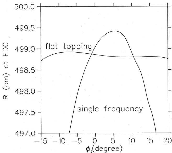
Fig. 1 Radial beam spread at the entrance of the EDC as a function of starting rf phase for single frequency and flat topping cases.
