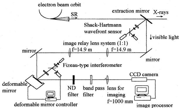
Fig.2 The design of adaptive optical system for the monitor
