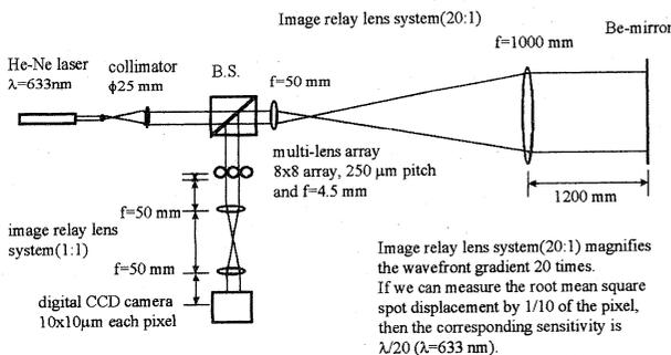
Fig.3 Outline of the Shack-Hartmann wavefront sensor.
