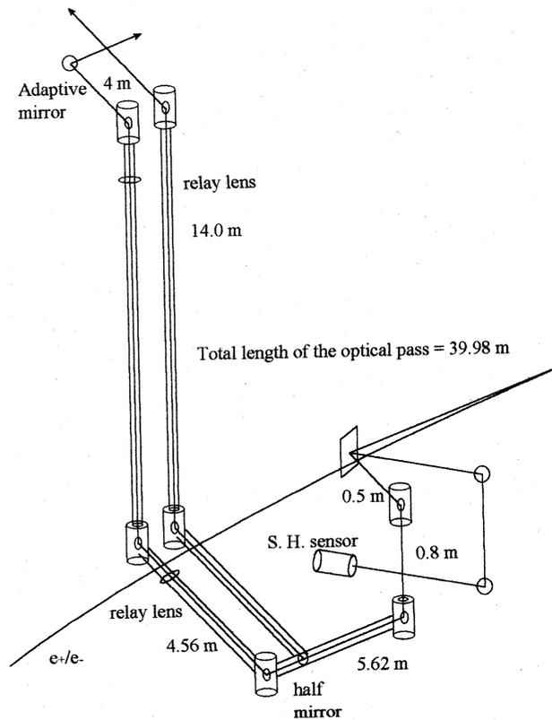
Fig.1 Outline of the SR-interferometer.
