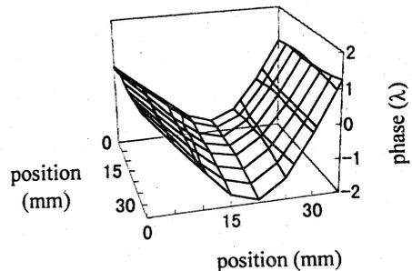
Fig.4 A result of the measurement of a wavefront error caused by SR-extraction mirror at BL-27
