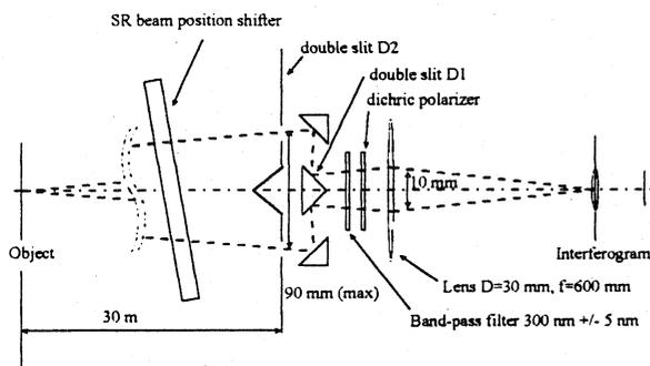
Fig.5 A design of SR-interferometer for B-factory.
