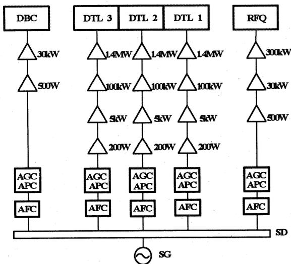
Fig. 3 Block diagram of RF system.
