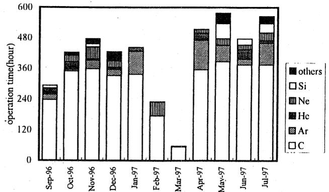
Fig. 1 Operation time of HIMAC injector.
