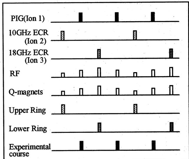
Fig. 4 Time chart in TSA operation. RF and Q-magnets show the excitation level, and the others show the beams.
