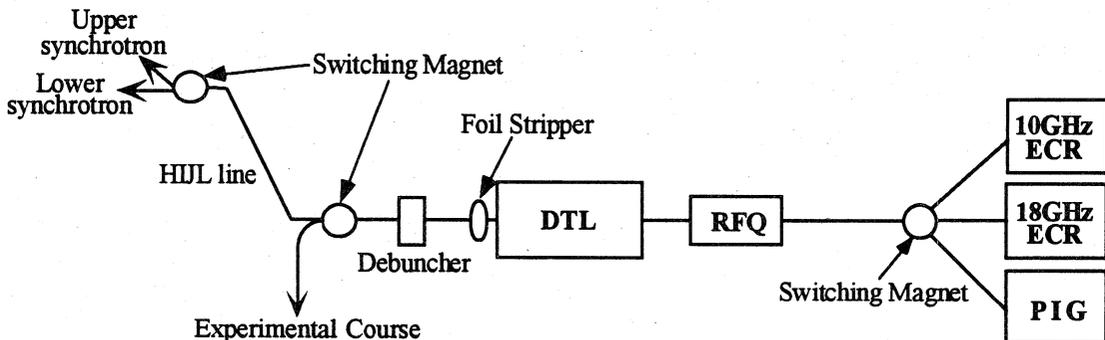
Fig. 2 Schematic drawing of the HIMAC injector, including the HIJL line.
