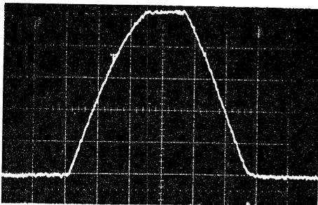
Fig. 5 Switching characteristics of the pulsed switching magnet for ion sources.  $T_{\text{rise}}$  and  $T_{\text{fall}}$  are 45ms.
