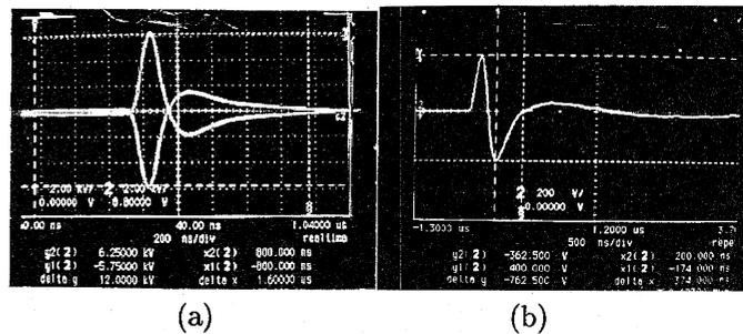
Figure 6: (a) An isolated pulse of 10kV in class B operation. Each waveform shows the voltage between either sides of the gap and earth. (b) An isolated pulse in class AB operation.
