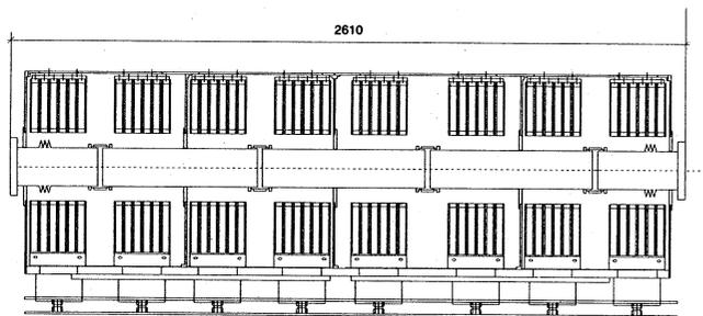
Figure 5: Schematic cross section of the modified cavity.
