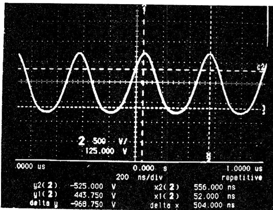
Figure 4: Waveform of the voltage in class AB operation.
