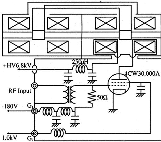
Figure 1: Schematic view of 30kW amplifier and test cavity.
