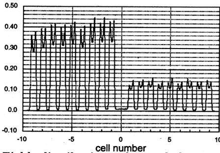
Fig. 6 Field distribution of no choke termination ( $f_a=2857$ [MHz],  $f_c=3029$ [MHz])
