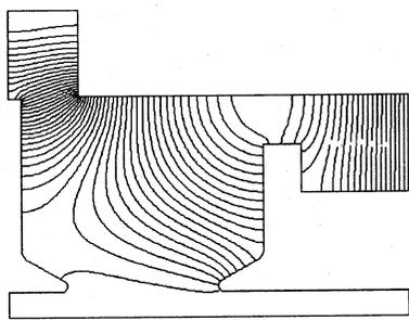
Fig. 4 The electric field of the coupling mode.
