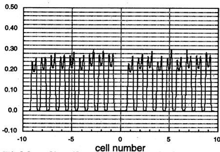
Fig. 7 Field distribution of choke termination ( $f_a=2854$ [MHz],  $f_c=2857$ [MHz])
