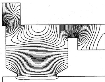
Fig. 3 The electric field of the accelerating mode.
