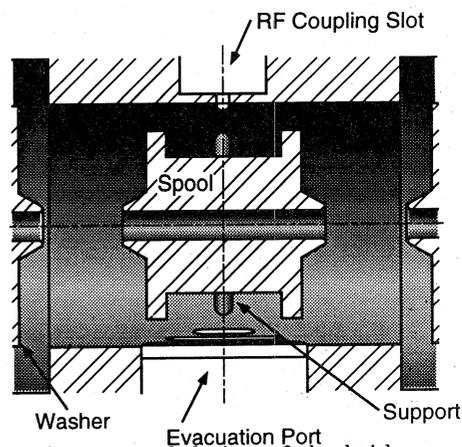
Fig. 2 Conceptual design of the bridge coupler
