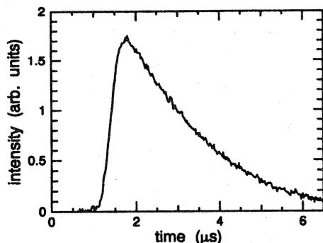
Fig. 3 The time spectrum of the laser light from the FEL operated at the wavelength 129  $\mu\text{m}$  measured with the fast Ge:Ga detector.
