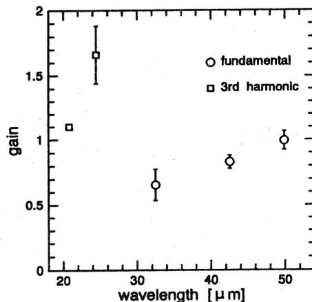
Fig. 1 FEL gain as a function of the wavelength below  $50\ \mu\text{m}$ . The data points denoted by the circles and the squares are assigned to the fundamental oscillation and third harmonic oscillation, respectively. See text for details.
