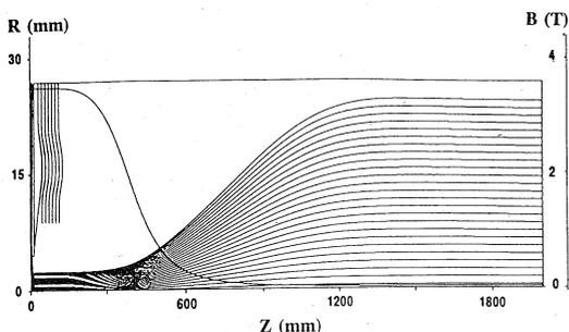
Fig. 2 Axial magnetic field and typical electron trajectories in the electron gun region at an energy of 2.5 keV and a current of 0.1 A.
