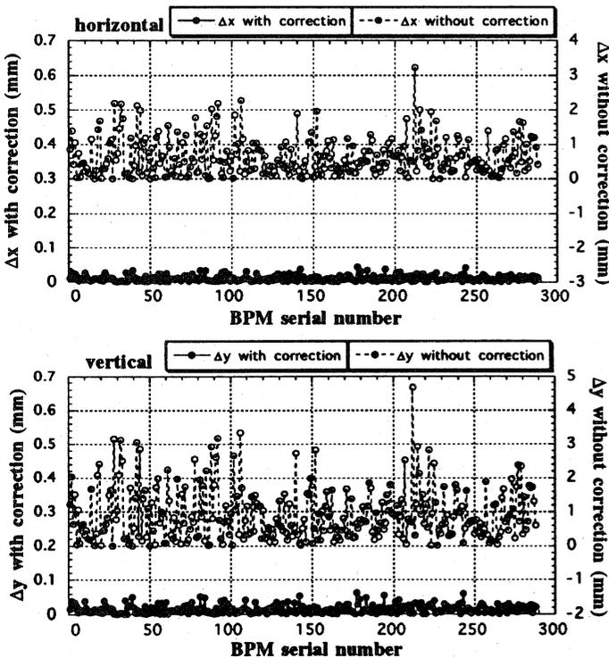
Figure 3 The comparisons between  $\Delta x$ ,  $\Delta y$  with and without the corrections by parameters  $f_2$ ,  $f_3$ ,  $f_4$ .
