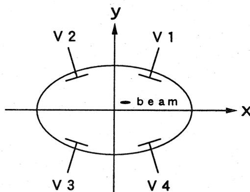
Figure 1 Schematic view of a BPM with four electrodes and the coordinate system.
