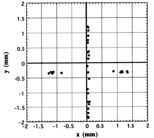
Figure 2 Typical distribution of beam positions at a BPM. There are 36 points.
