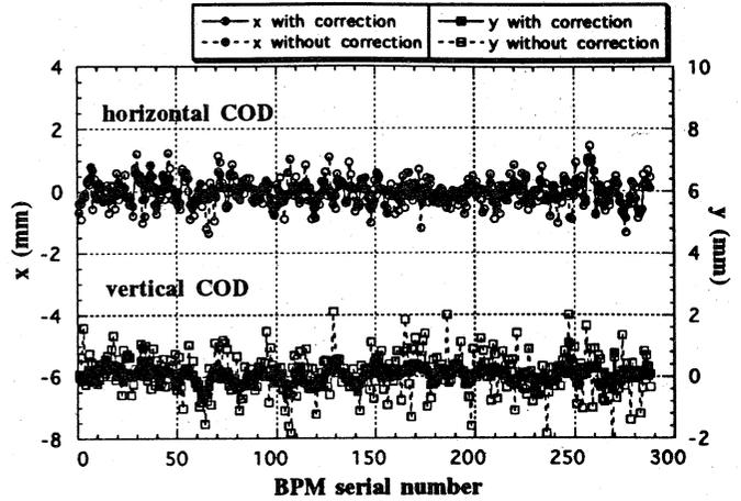
Figure 4 The comparison between CODs with and without the corrections by parameters  $f_2$ ,  $f_3$ ,  $f_4$ .
