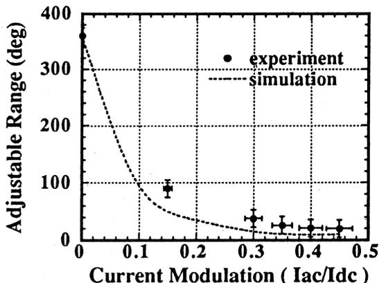
Fig.7 Adjustable range of the output microwave phase by changing the input microwave phase.
