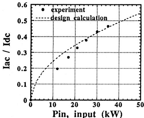
Fig.3 Current-modulation attained at the wiggler entrance.
