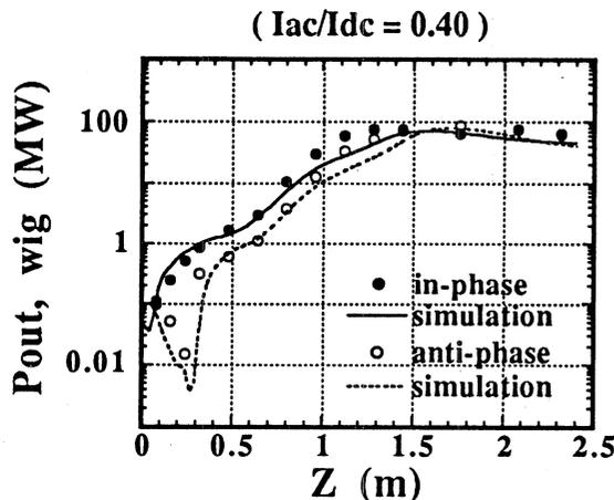
Fig.5 Microwave power evolutions in the case of stimulated operation.
