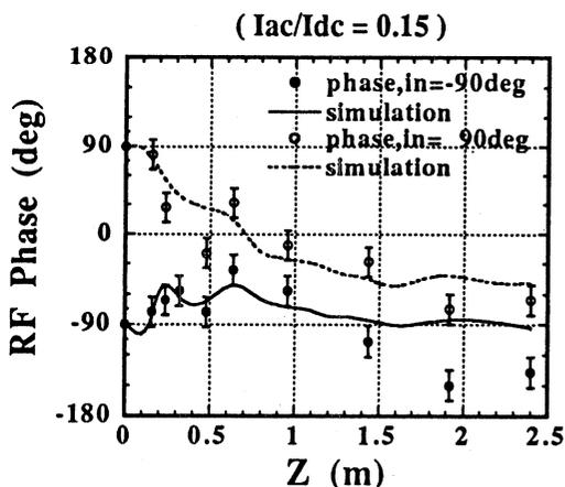
Fig.6 Microwave phase evolutions for different initial phases of the input microwave. The zero phase is when the beam bunch-center is located at the maximum decelerating field of the input microwave.
