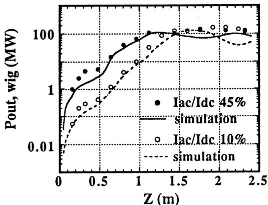
Fig.4 Microwave power evolutions in the case of superradiant operation.
