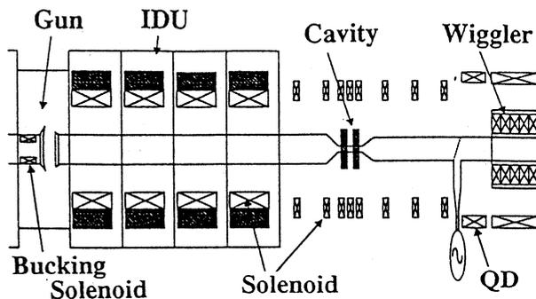
Fig.1 Configuration of the prebunched FEL amplifier.
