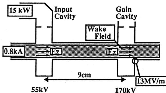
Fig.2 Prebunching cavities.
