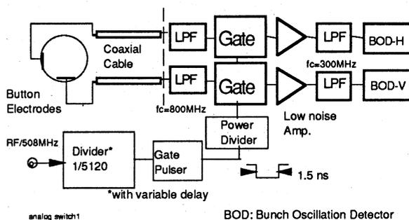
Fig. 4 Block diagram for detecting the betatron tunes.
