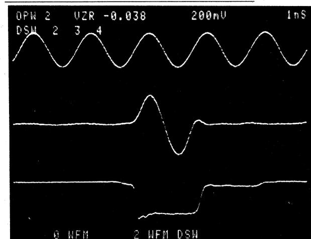
Fig. 3 Transient response of the switch. Upper trace shows an input rf signal of 500MHz with 400mV/div. Middle one is a gated output signal with 50 mv/div. A low-pass filter of 800 MHz is used. Lower one is a gate pulse with 1V/div. All traces are swept with 1ns/div.
