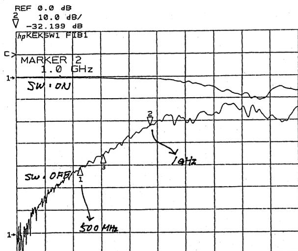
Fig. 2 Frequency characteristics. Horizontal frequency range is 0.05 GHz to 2.05 GHz. Vertical scale is 10dB/div.
