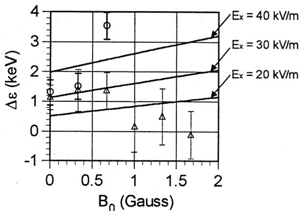
Fig.4. Energy increment,  $\Delta\varepsilon$ , as a function of the static magnetic field  $B_0$  with  $P = 10$  kW. The solid lines show the calculated values when  $E_0 = 20, 30$  and 40 kV/m. Symbols  $\circ$  and  $\triangle$  stand for  $\varepsilon_0 = 64$  keV and 66 keV, respectively.
