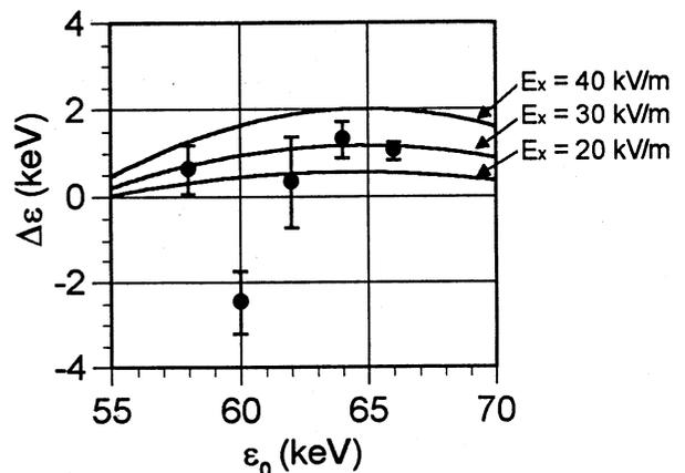
**Fig.3.** Energy increment,  $\Delta\epsilon$ , as a function of the incident electron energy,  $\epsilon_0$ , without external magnetic field. Incident microwave power:  $P = 10$  kW. The solid lines indicate the calculated maximum energy increment, at the maximum electric field value of  $E_x = 20, 30$  and  $40$  kV/m.
