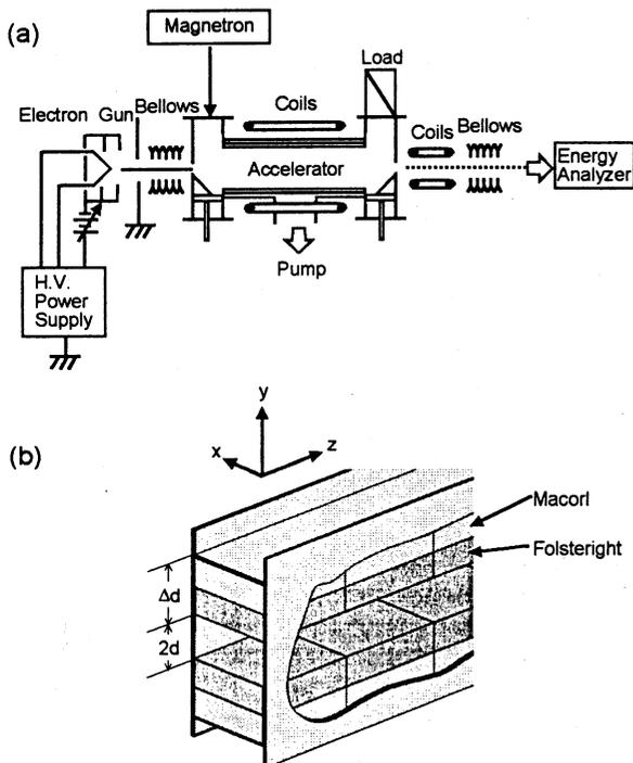
**Fig.2.** Experimental apparatus and the crosssectional view of the wave guide loaded dielectric material. (a) Experimental apparatus for the proof of the principle of the electron accelerator using TE wave. (b) Schematic drawing of the dielectric wave guide.
