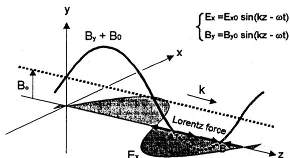
Fig.1. Schematic diagram of the  $v_p \times B_0$  acceleration using a transverse electromagnetic wave. An electromagnetic wave with a transverse electric field component propagates in the  $z$  direction with the phase velocity  $v_p$ . A static magnetic field  $B_0$  is applied in the  $y$  direction. A charged particle is accelerated in the  $x$  direction.
