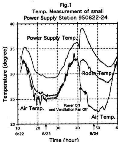
It will be able to keep the room temperature in the range of 20 to 40 degrees in all the year only by on/off control of ventilation fan. Consequently it became clear that to guarantee the specification given in Table 1 the design of KEKB magnet power supplies must be carried out by taking account of the room temperature change of 20 degrees.
