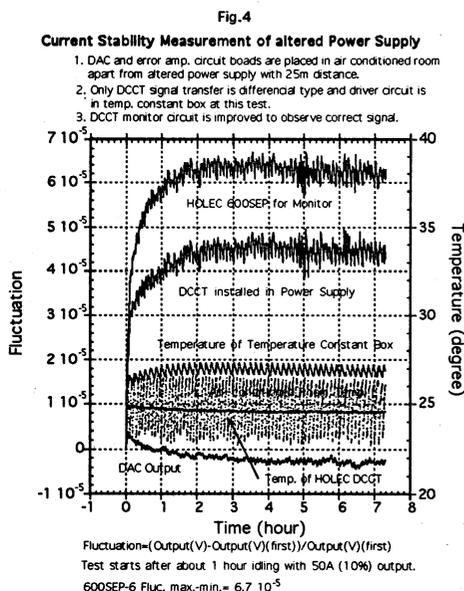
The current stability of this power supply is within 10 ppm after warming up. This value is enough for the specification of KEKB magnet power supplies.
