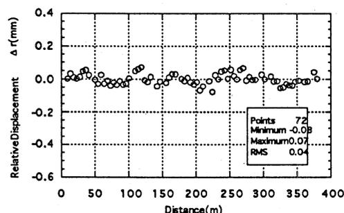
Fig. 3. Relative displacement between girders.
