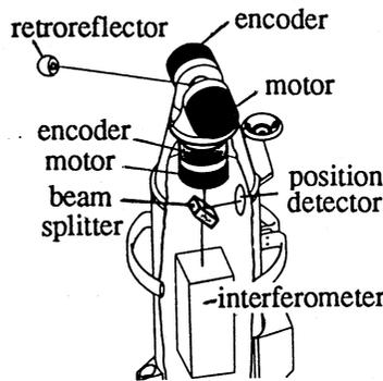
Fig.1 Principle of the laser tracker
