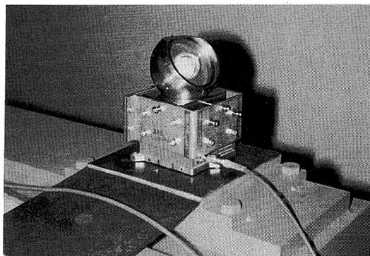
Fig.4. Tiltmeter and SMART target on it.
