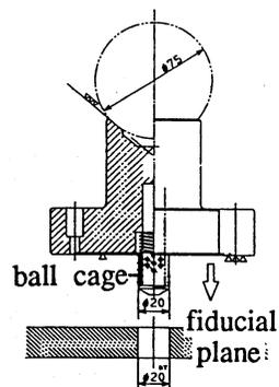
Fig. 7. Stage on which the target is put.
