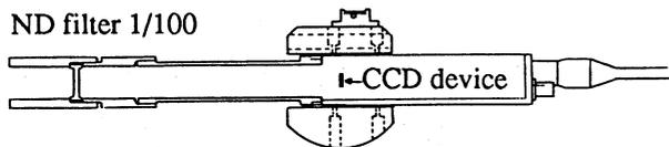
Fig. 6. CCD camera with spherical housing.
