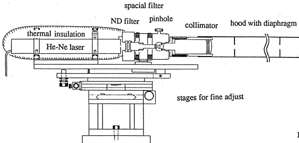
Fig. 5. Laser with spacial filter and collimator.
