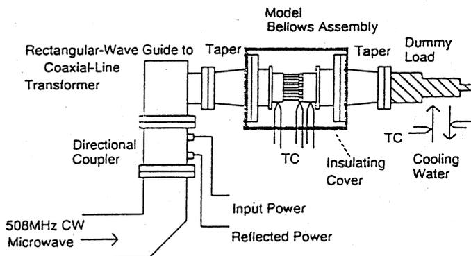
Fig.3. A schematic diagram of experimental apparatus
