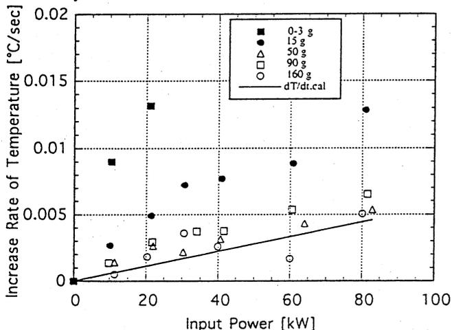
Fig.4. The increase rate of temperature (°C/sec) versus input microwave power. The straight line is the calculated minimum increase rate of temperature.
