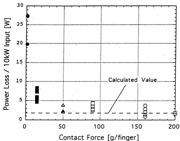
Fig.5. The power loss per 10 kW input power versus the average contact force. The dotted line is the calculated minimum power loss.
