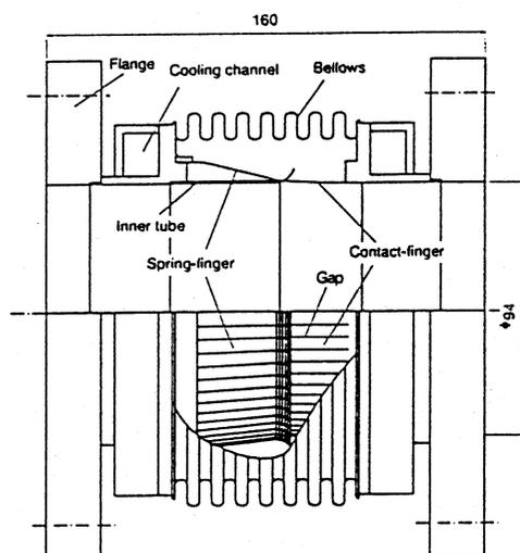
Fig.1. A schematic drawing of the bellows assembly
