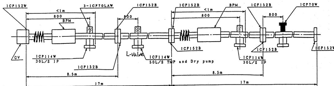
Fig.5 A prototype beam chamber consists of dummy beam position monitors, pumping ports, gauge ports and bellows.
