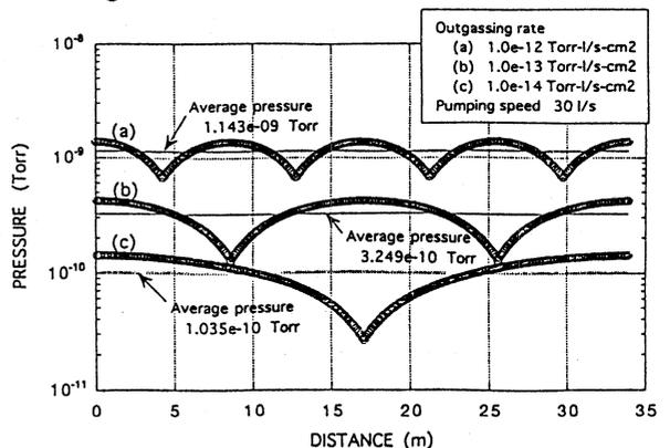
Fig.4 Pressure distribution along the beam chamber.
