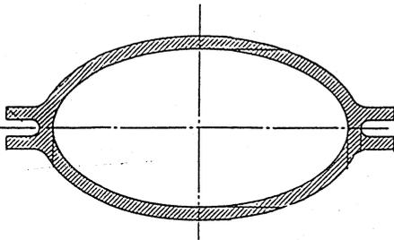
Fig.1 Cross section of beam chamber for bending and quadrupole magnets.
