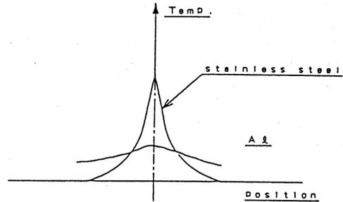
Fig.2 Temperature distribution irradiated from localized high heat flux against stainless steel and aluminum.
