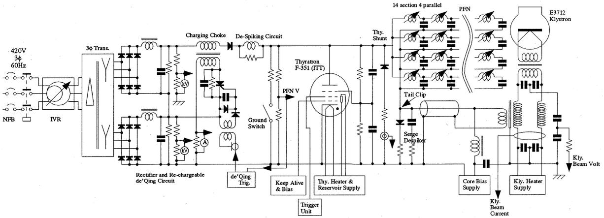
Fig.1 Outline of the modulator circuit
