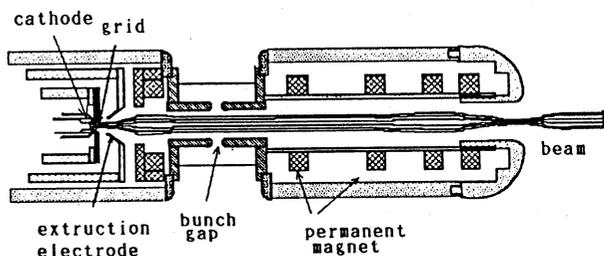
Fig.2 Cross sectional view of the stem with a beam focusing system and a buncher.
