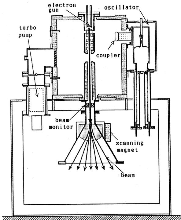
Fig.6 Cross sectional view of ES for industrial use.
