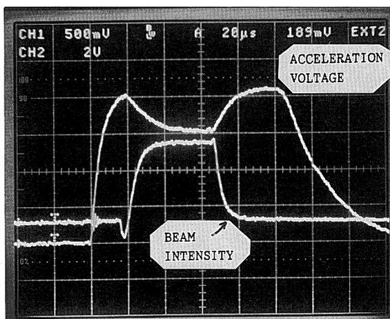
Fig.3 Typical beam loading effect.
