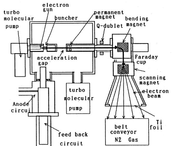
Fig.1 Cross-sectional view of ELECTRON SHOWER.
