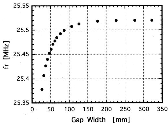
Fig. 3 Characteristics of the capacitive tuner.
