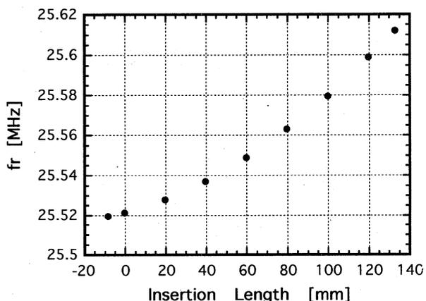
Fig. 2 Characteristics of the adjustable reactive-tuner.
