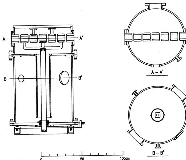
Fig.1 Cross section of the 25.5 MHz rebuncher.
