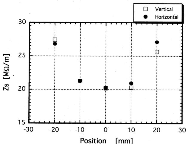
Fig. 5 On- and off-axis shunt-impedances. The horizontal and the vertical positions are measured from the drift tube center to the capacitive tuner, and to the upper direction, respectively.
