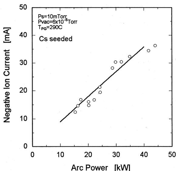
Fig.2 Negative ion beam as a function of arc discharge power
