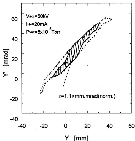
Fig.3 Emittance diagram at an acceleration voltage of 50 kV
