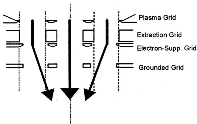
Fig.4 A conceptual illustration of the multi-aperture displacement technique
