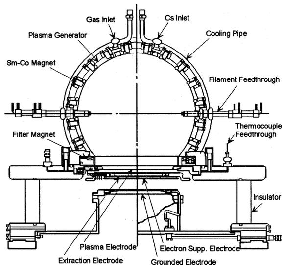
Fig.1 Cross sectional view of the negative ion source
