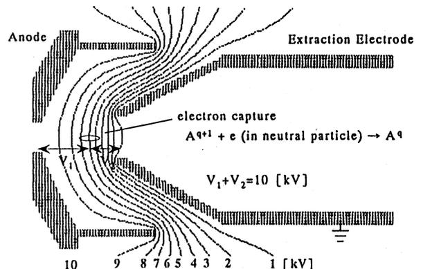
Fig.5. one electron capture in acceleration gap
