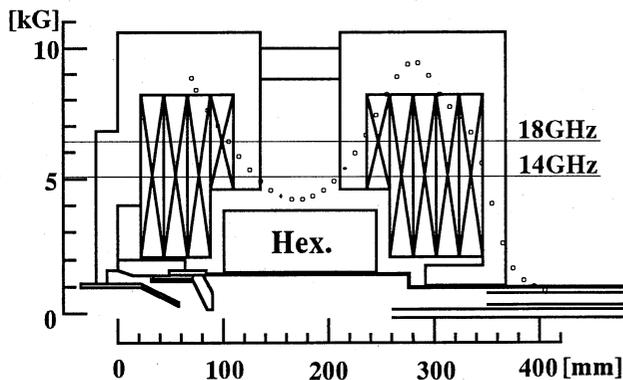
Fig.3. axial mirror field distribution(mirror coils current 600 [A])
