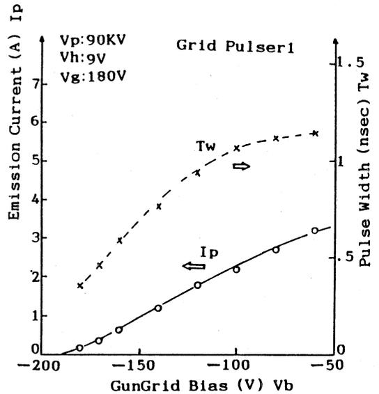
Fig. 3. Relation between grid bias and emission current (Pulser I).
