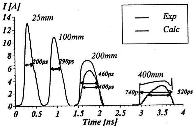
Fig. 7. Bunch lengthening calculated based on the disk model.
