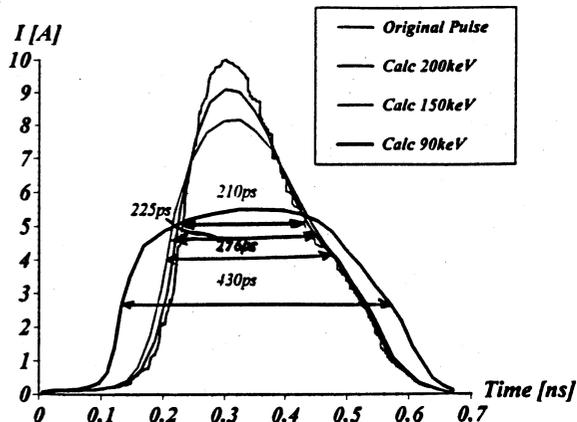
Fig. 8. Dependence of bunch lengthening on accelerating voltage.
