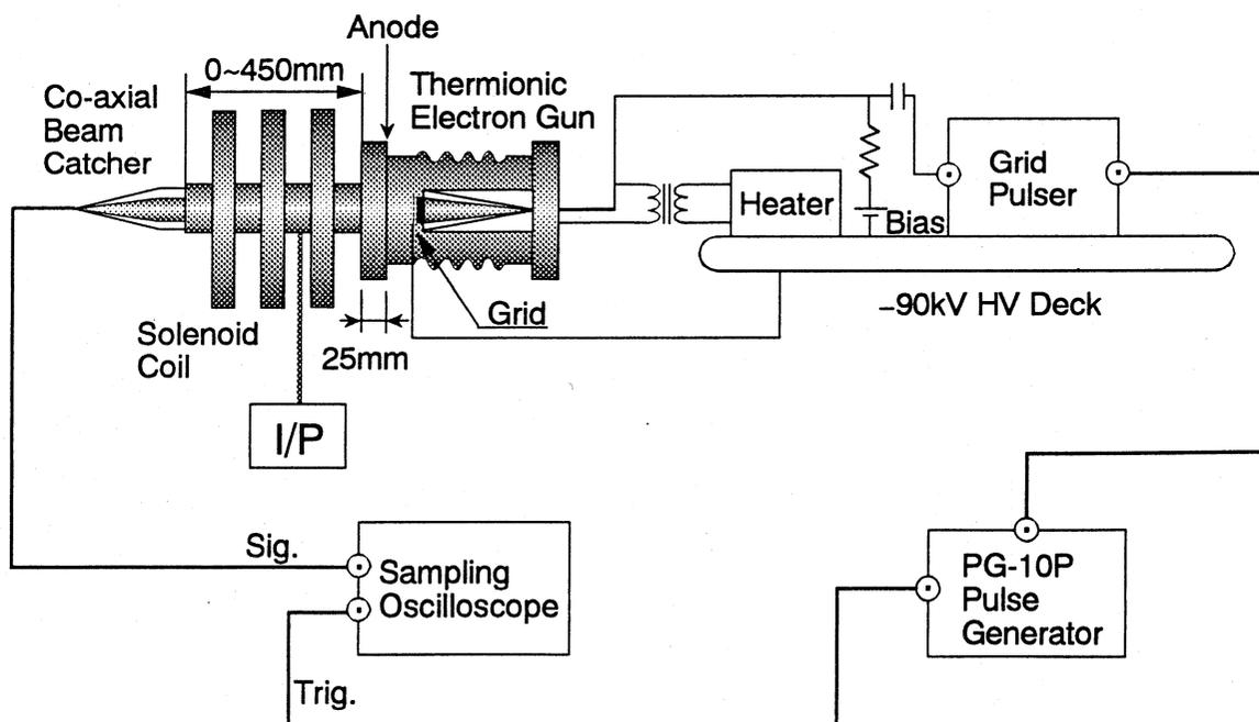
Fig. 1. Test bench for an thermionic electron gun.
