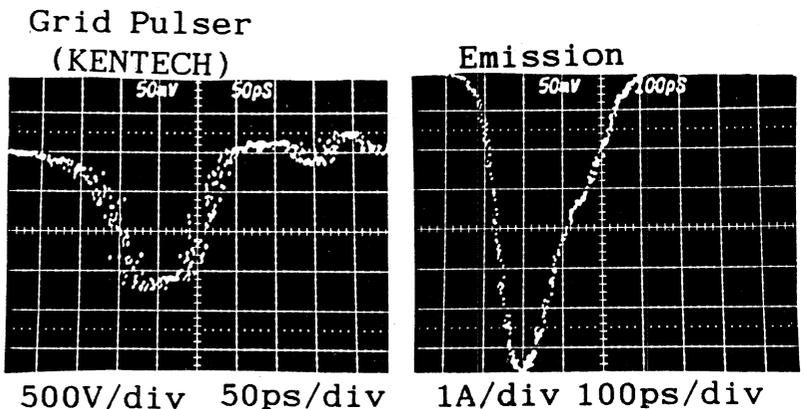
Fig. 4. Typical output waveforms of Pulser II and of the emission at the distance of 25 mm.
