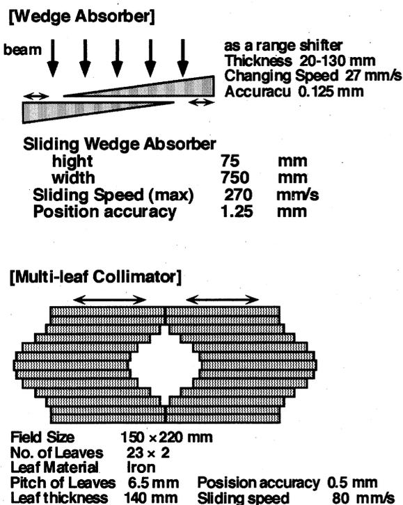
Figure 3: Specification of wedge absorber and multi-leaf collimator.
