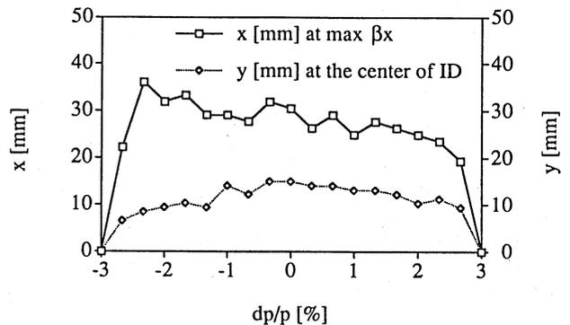
Fig. 5 Horizontal and vertical dynamic apertures versus momentum deviation
