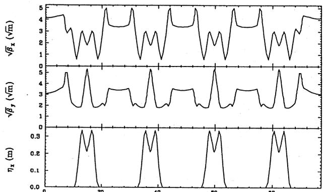
Fig. 4 Optics of a superperiod
