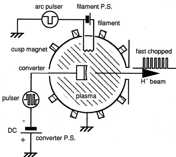
Fig.1: The schematic drawing of the surface-plasma  $H^-$  ion source.
