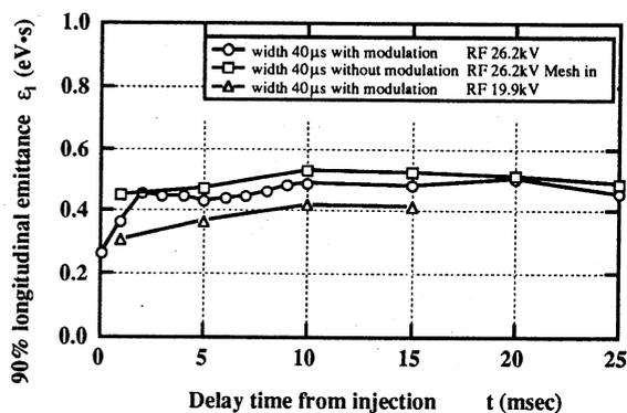
Fig.5: The longitudinal emittance as a function of the injection time.
