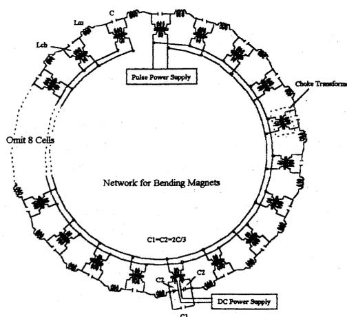
Fig. 3 Schematic view of the BM Network.
