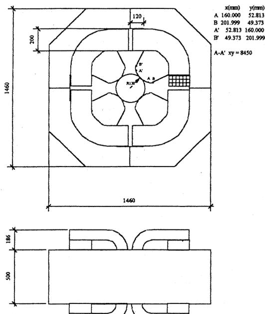
Fig. 2 Plan view of the quadrupole magnet.
