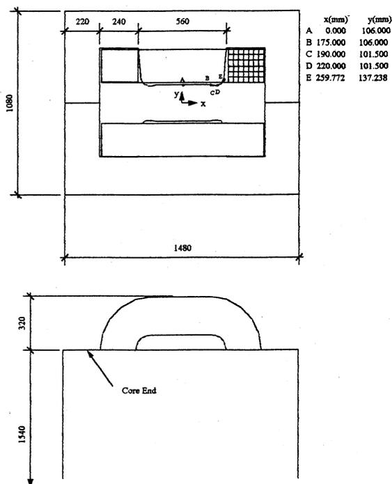
Fig. 1 Plan view of the bending magnet.
