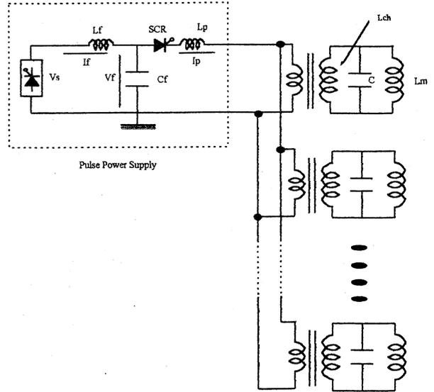
Fig. 4 Schematic view of the pulse power supply.
