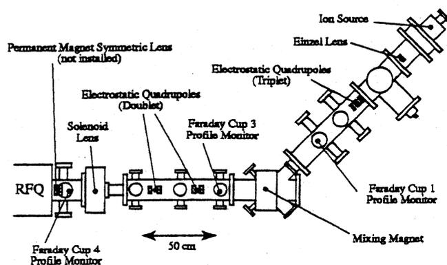
Fig. 1. The injection line of the proton linac
