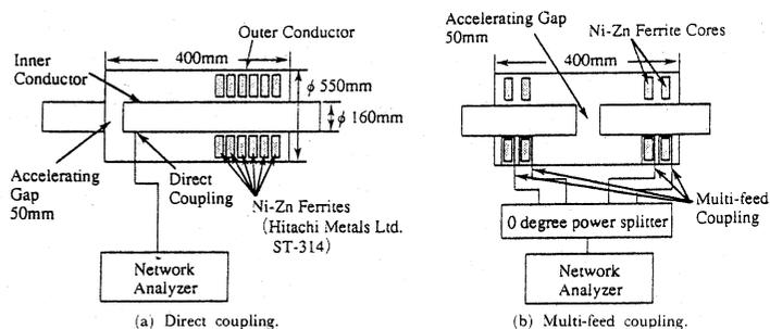
**Fig. 7. Setup of the direct and multi-feed coupling**
