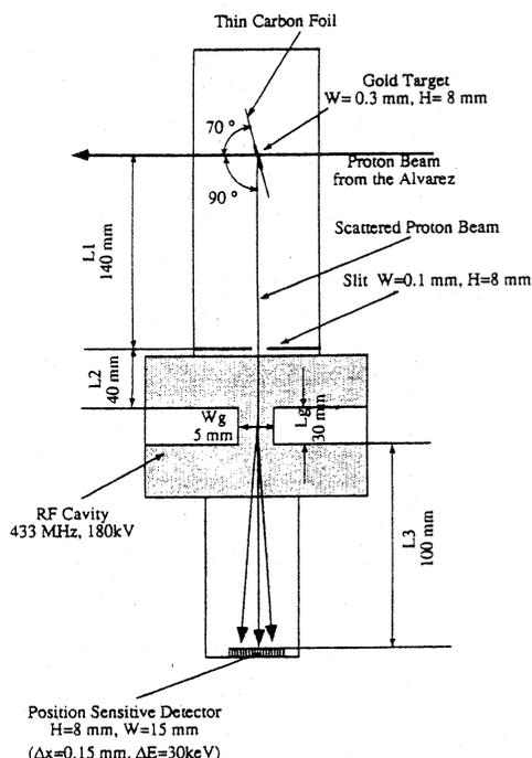
Fig. 3. Concept of the longitudinal emittance monitor
