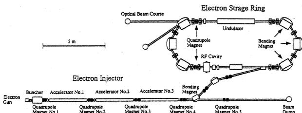
Fig. 4. Layout of the electron linac and the storage ring KSR
