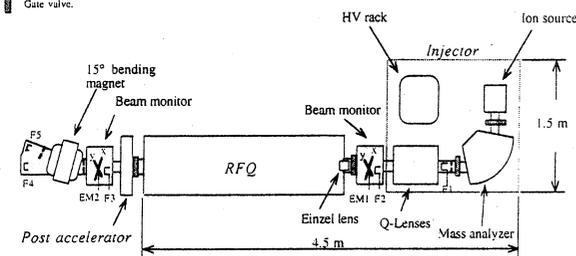
**Fig. 6. Experimental setup of the 4-rod RFQ linac system**
