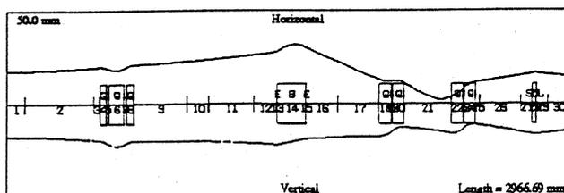
Fig. 2. The matched beam envelope between einzel lens and PMS section at current of 20mA (TRACE-3D calculation).
