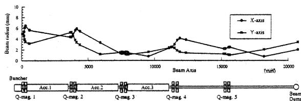
Fig. 5. Calculated beam radius (emittance of 100πmmrad)
