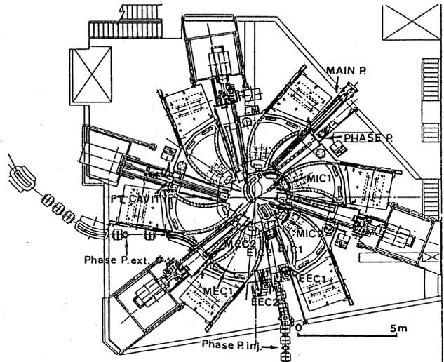
Fig.1 Plan view of the ring cyclotron.
