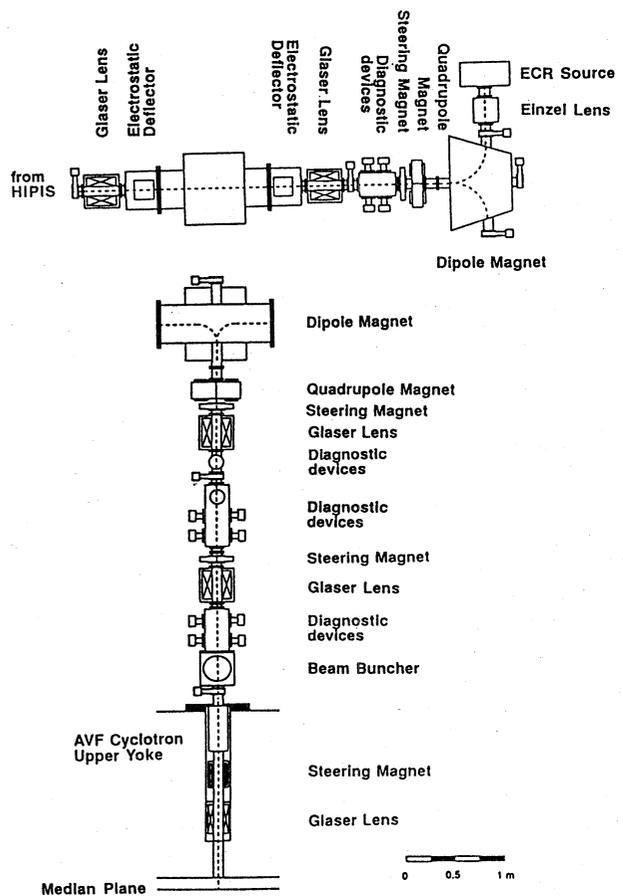
Fig.2 Layout of the injection line.
