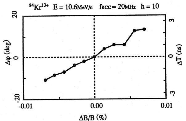
Fig.3 The peak shift (that is, beam phase) vs the change of magnetic field in the RRC.
