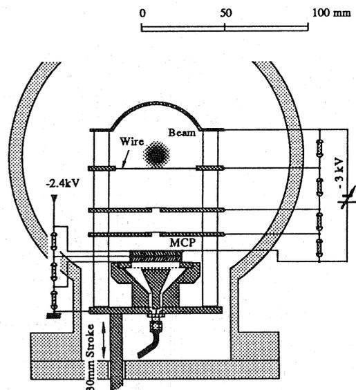
Fig. 1. A structure of a new type of beam phase monitor with an MCP. All electrodes are made of stainless steel and supported by ceramic insulator rods. Each electrode is biased so that a uniform field is produced from the wire to the MCP.
