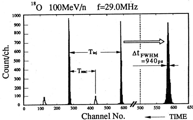
Fig. 2 Example of time spectrum of signals from the MCP for a 100MeV/n  $^{18}\text{O}$  beam. These signals are considered to originate from photons produced at the wire by the beam, because no acceleration voltage is applied of the electrode during this measurement. A start signal for the TAC is given by the MCP signal and a stop signal is an rf reference. Shaded peaks are due to a main beam, and unshaded peaks are due to the effect of multi-turn extraction.
