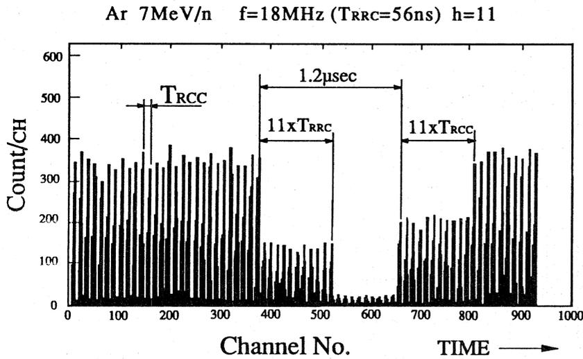
Fig. 4. A time spectrum of beam bunches when the beam is cut partially ( $1.2\mu\text{s}$ ) by the beam chopper installed in the RILAC injection line. The start of the TAC is done by the trigger signal for the chopper, which is synchronized to the rf phase. The stop for the TAC is the MCP signal.
