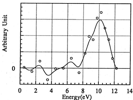
Fig.3 Energy Spread of Input 10eV Beam
