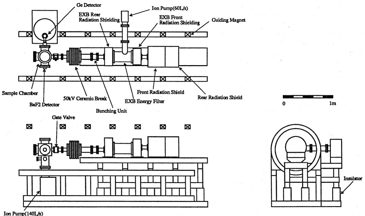
Fig.1 Schematic Diagram of Slow Positron Beam System
