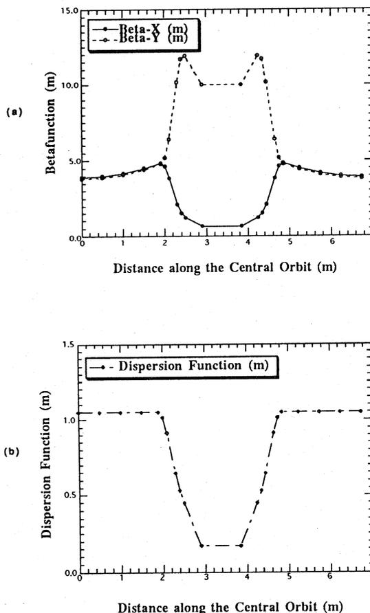
Fig. 3 Betafunctions (a) and dispersion function (b) in a quadrant of the ring.
