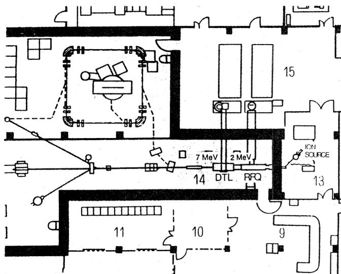
Fig.1 Layout of the proton linac and the proposed ring
