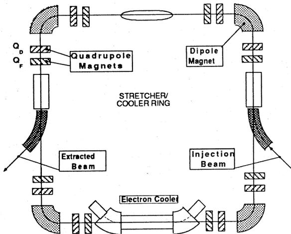
Fig. 2 Layout of the Arrangement of the stretcher/cooler ring
