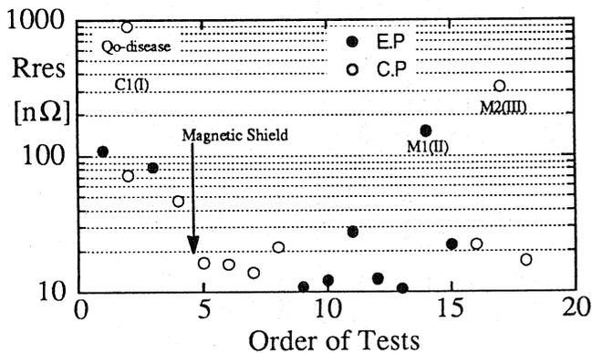
Fig. 3 Residual surface resistances for each test.
