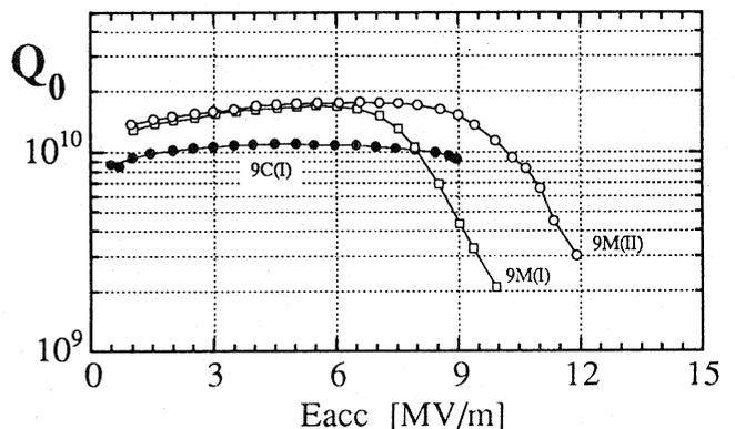
Fig. 5  $Q_0$  -  $E_{acc}$  plots for the 9-cell cavities.
