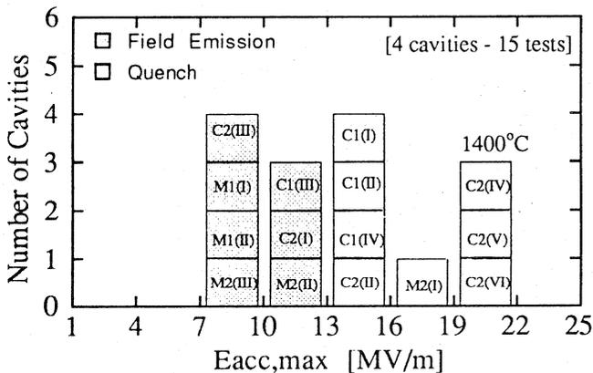
Fig. 2 Distribution of the  $E_{acc,max}$  for 15 tests on 4 single-cell cavities.
