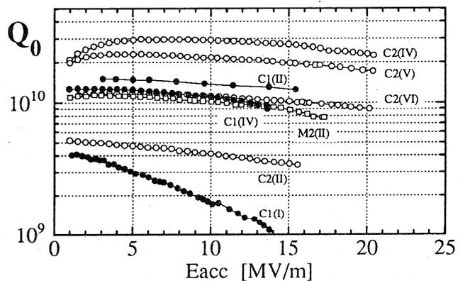
Fig. 4  $Q_0$  -  $E_{acc}$  plots in the case of no  $Q_0$ -drop by field emission for the single-cell cavities.
