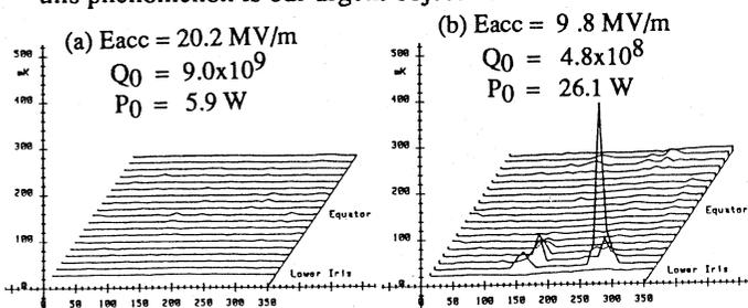
Fig. 6 Temperature mapping [Test: C2(VI)]; (a) at just below Eacc,max before quenching, and (b) in the strong electron loading region after quenching at Eacc,max.
