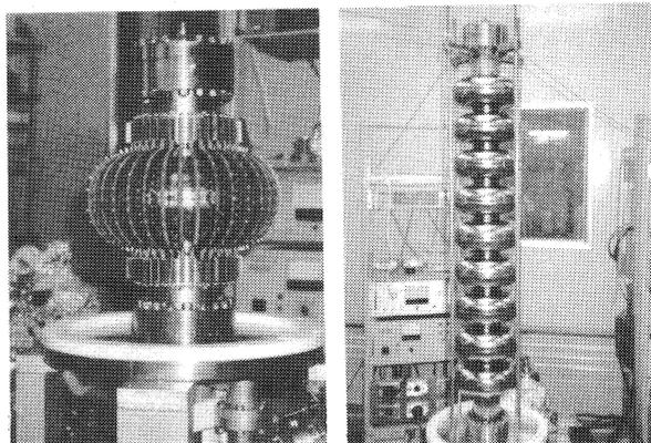
Fig. 1 A single-cell cavity with attached carbon thermometers (left) and a 9-cell cavity (right) installed in the vacuum stand.
