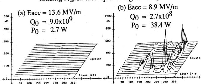
Fig. 7 Temperature mapping [Test: C1(IV)].
