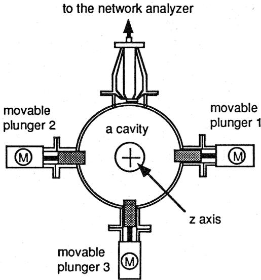
Figure 2. A schematic diagram of the multi-plunger system.
