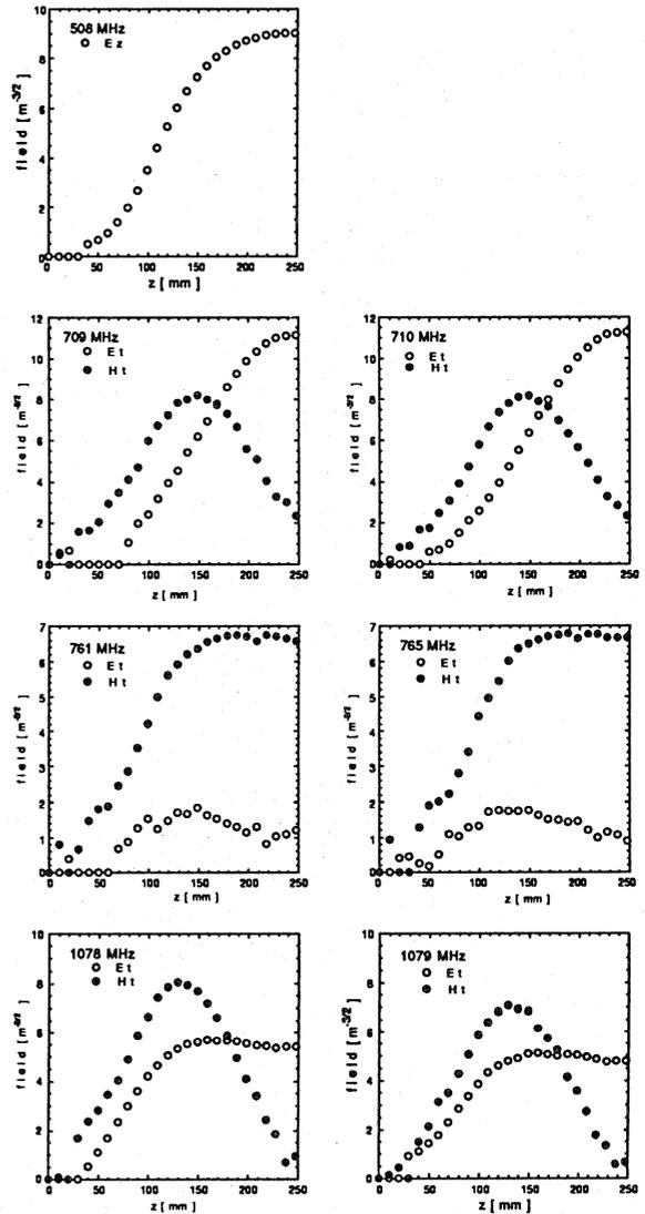
Figure 3. Field distributions of the accelerating mode (508.58MHz) and dipole higher order modes from the entrance of the cavity to the center. Ez means electric field parallel to the beam axis (the z-direction) and Et and Ht stand for transverse electric and magnetic fields, respectively.
