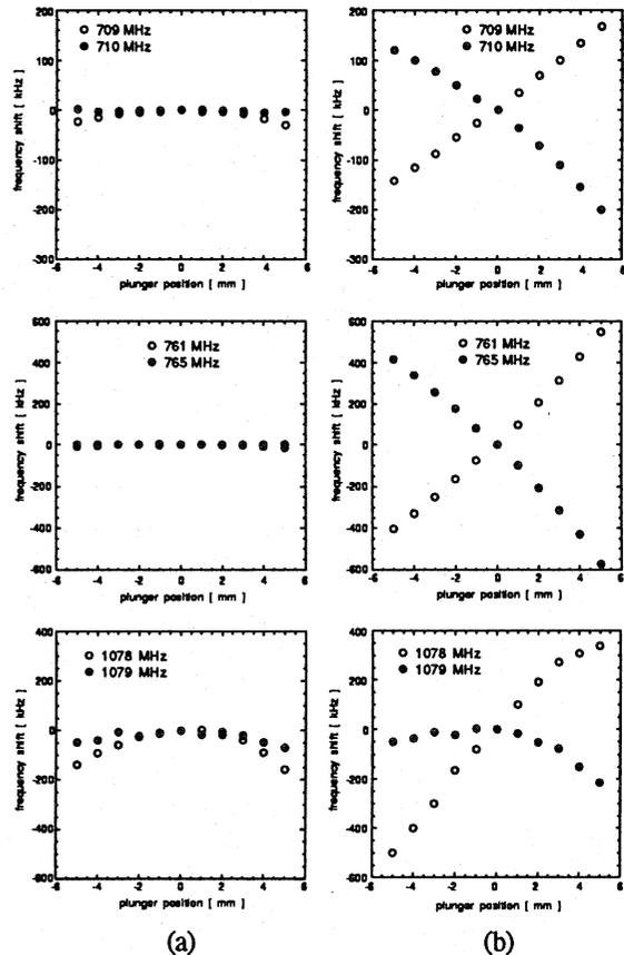
Figure 5. Results of frequency shifts of higher order modes with a diagram of two movable plunger system. (a) two plungers were set on both horizontal sides of the cavity (the plunger 1 and the plunger 2 were used) and (b) one was set on the horizontal side and the other was set on the vertical lower side (the plunger 1 and the plunger 3 were used).
