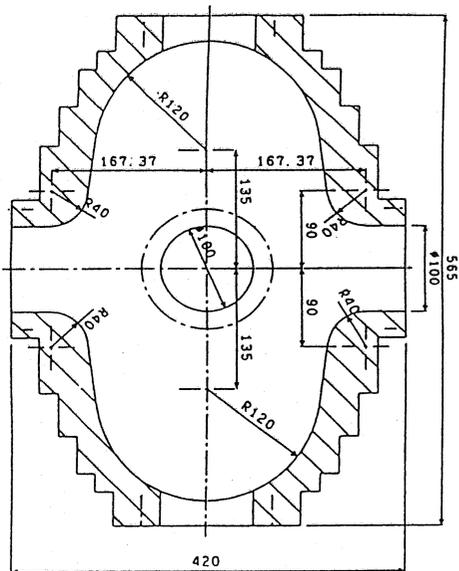
Figure 1. Cross section of a bell shaped single cell cavity.
