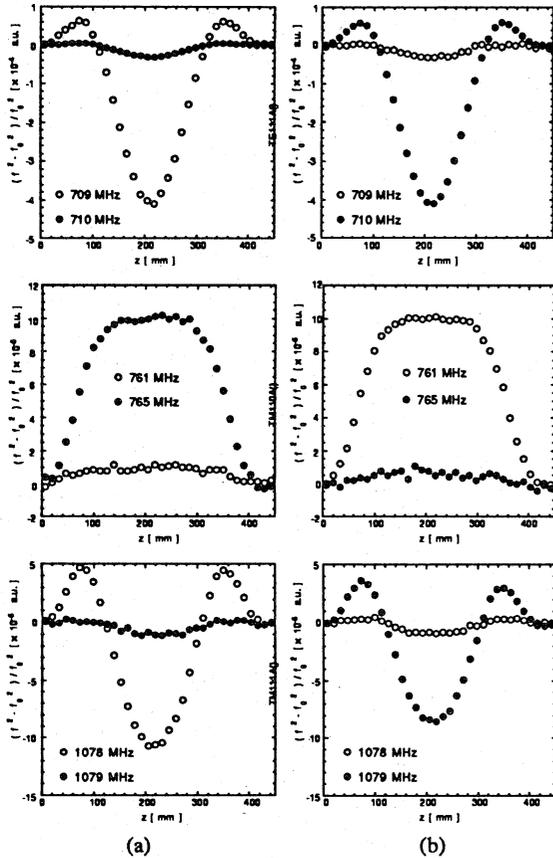
Figure 4. Frequency shifts of dipole HOMs by the rectangle copper plate directed (a) horizontally and (b) vertically.
