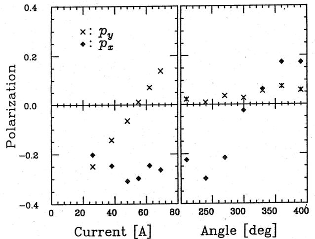
Fig.4. Polarization measured at the exit of the AVF cyclotron ( $E_d = 14$  MeV) by using the  $^{12}\text{C}(d,p)^{13}\text{C}_{\text{gnd}}$  reaction by varying the current and the angle of the spin rotator.
