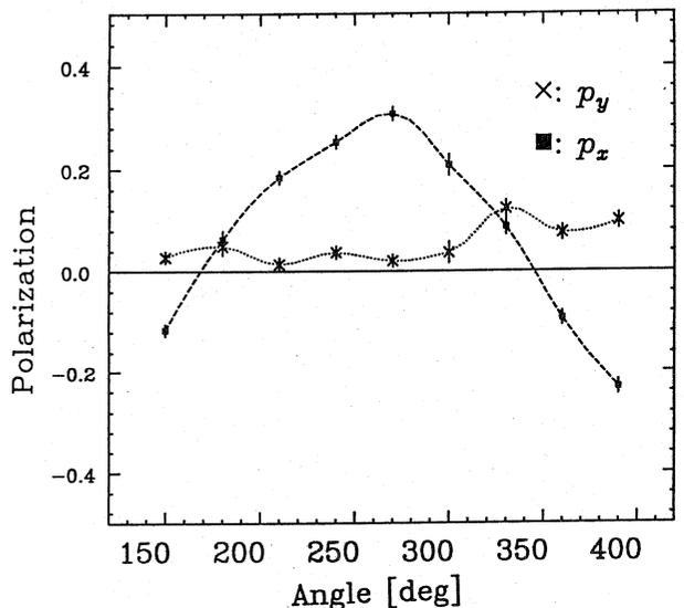
Fig.5. Polarization measured at the exit of the ring cyclotron ( $E_d = 270$  MeV) by using the  $d + p$  elastic scattering by varying the angle of the spin rotator.
