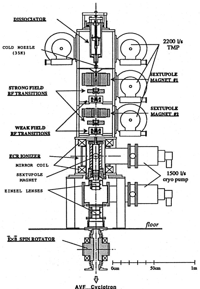
Fig. 1. Side view of the polarized ion source.
