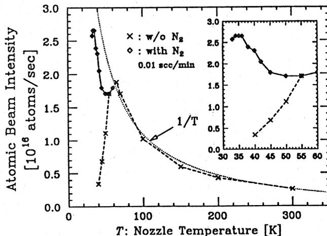
Fig.2. Dependence of atomic beam intensity on the nozzle temperature.
