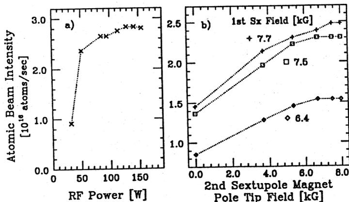
Fig. 3. Dependence of atomic beam intensity (a) on the dissociator RF power and (b) on the pole-tip field of the sextupole magnets.
