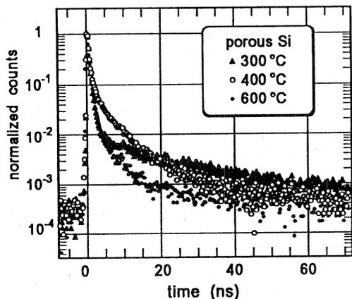
Figure 2. Positron lifetime spectra of porous Si at the sample temperatures of 300 °C, 400 °C, and 600 °C.
