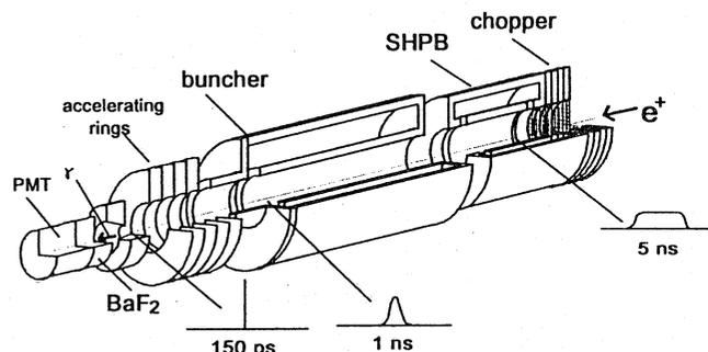
Figure. 1. The positron pulsing system.
