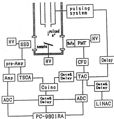
Figure 3. Block diagram of the AMOCS system.
