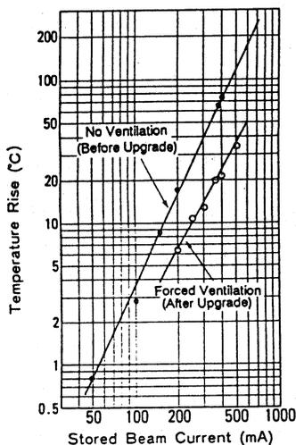
Figure 2. Temperature rise of the ceramic duct facing a bump magnet.
