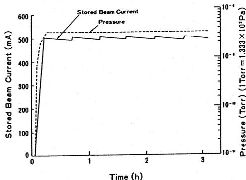
Figure 3. Constant control of the stored beam current.
