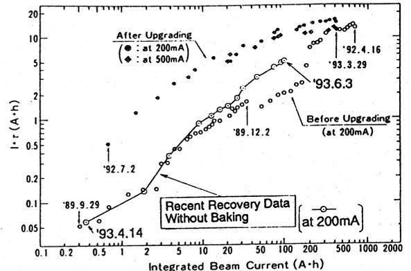
Figure 7. Improvement of beam lifetime as function of integrated beam current.
