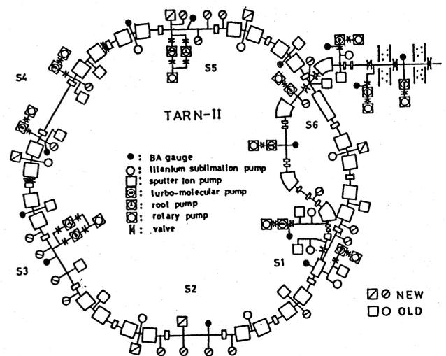
Fig. 1 Schematic layout of the vacuum system at TARN-II.
