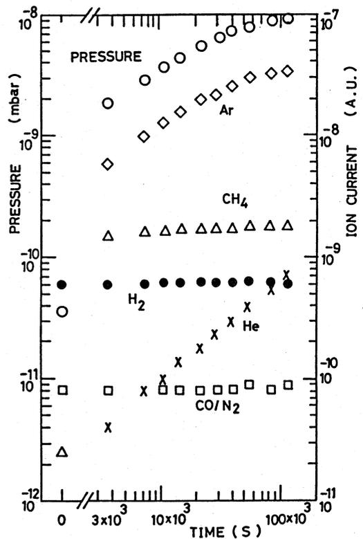
Fig. 5 Total pressure and residual gas as a function of time.
