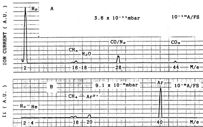
Fig. 4 Residual gas spectra of the ring.
