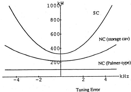
Figure 2. Necessary input power to maintain the accelerating voltage as a function of the tuning error.
