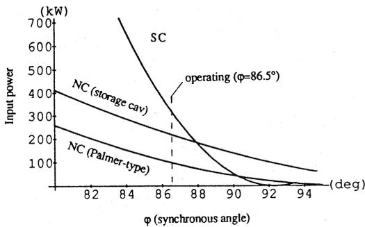
Figure 1. Necessary input power to maintain the accelerating voltage as a function of the phase error.
