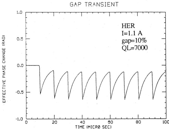
Figure 4. Modulation of bunch spacing in the case of 10 % gap in HER calculated with the transfer function.
