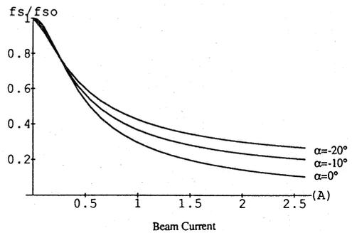
Figure 5. Change of coherent synchrotron frequency as a function of the beam current for the case of the Palmer-type cavity.  $\alpha$  is the phase difference between generator current and cavity voltage.
