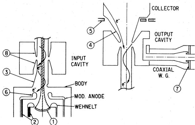
Fig. 2. Modifications against backstreaming electrons.
