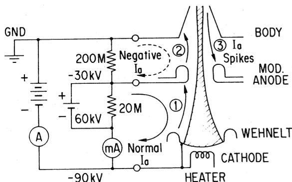
Fig. 1. Gun structure and potential level of each electrode.
