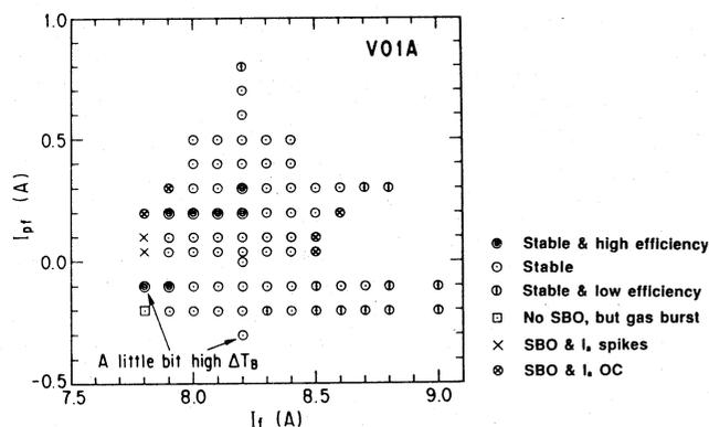
Fig. 4. A stability map vs. focusing & pre-focusing currents.
