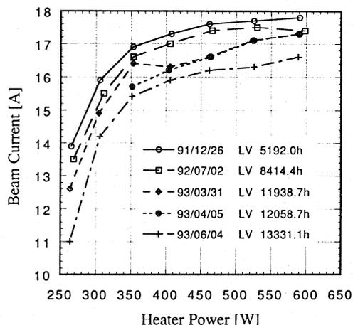
Fig. 3. Underheating data vs. time of V23.
