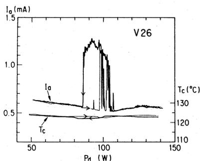
Fig. 5. Hysteresis of  $I_a$  and collector temperature  $T_c$  vs.  $P_d$ .
