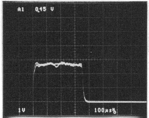
Figure 3. Observed beam pulse (output of a buffered amplifier) after the acceleration by Alvarez linac.
