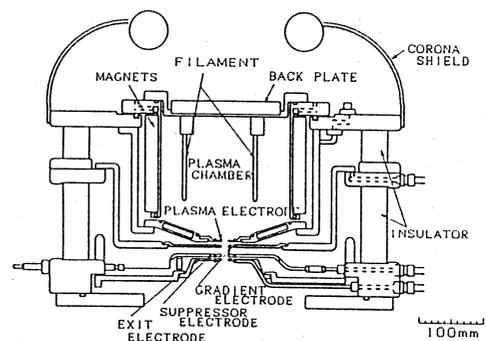
Fig. 1 Cross sectional view of the ion source
