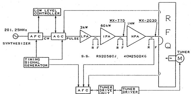
Fig. 8 Block diagram of the RF source
