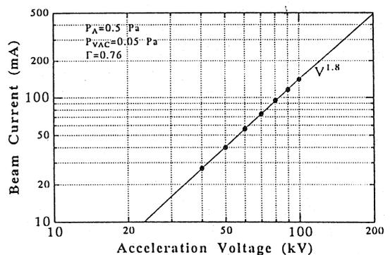
Fig. 2 Measured beam current as a function of acceleration voltage
