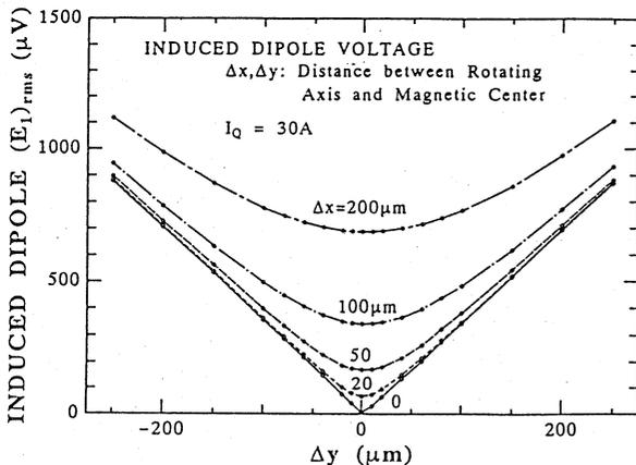
Fig. 6 Induced dipole voltage in the rotating coil as a function of the distance from the magnetic center  $\Delta y$  for five  $\Delta x$  case
