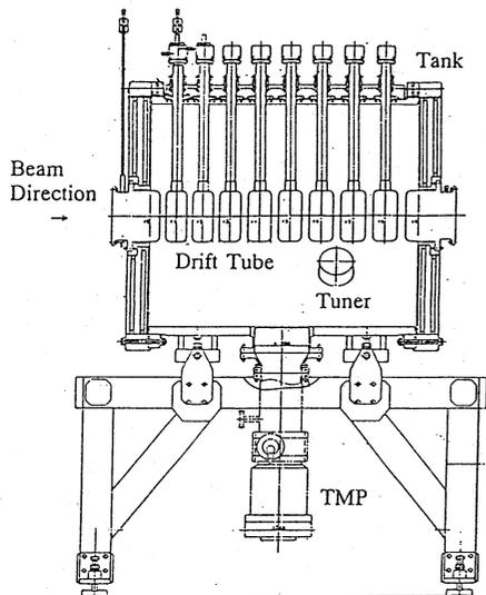
Fig. 7 Cross sectional view of the DTL high power model tank
