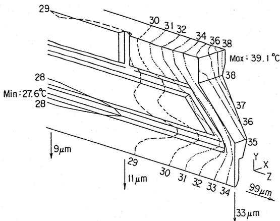
Fig. 3 Temperature distribution and displacement of the RFQ vane
