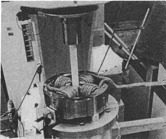
Fig. 5 Photograph of the quadrupole magnet and the rotating coil
